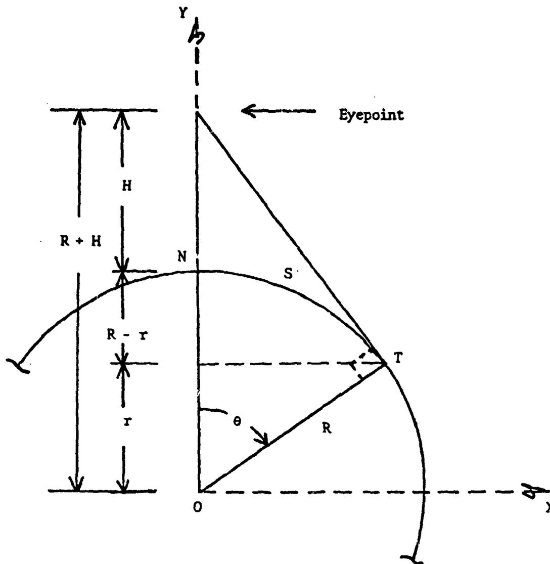
Figure 2.1.3.1-1. Visibility of Earth's Surface as a Function of Observer Altitude
