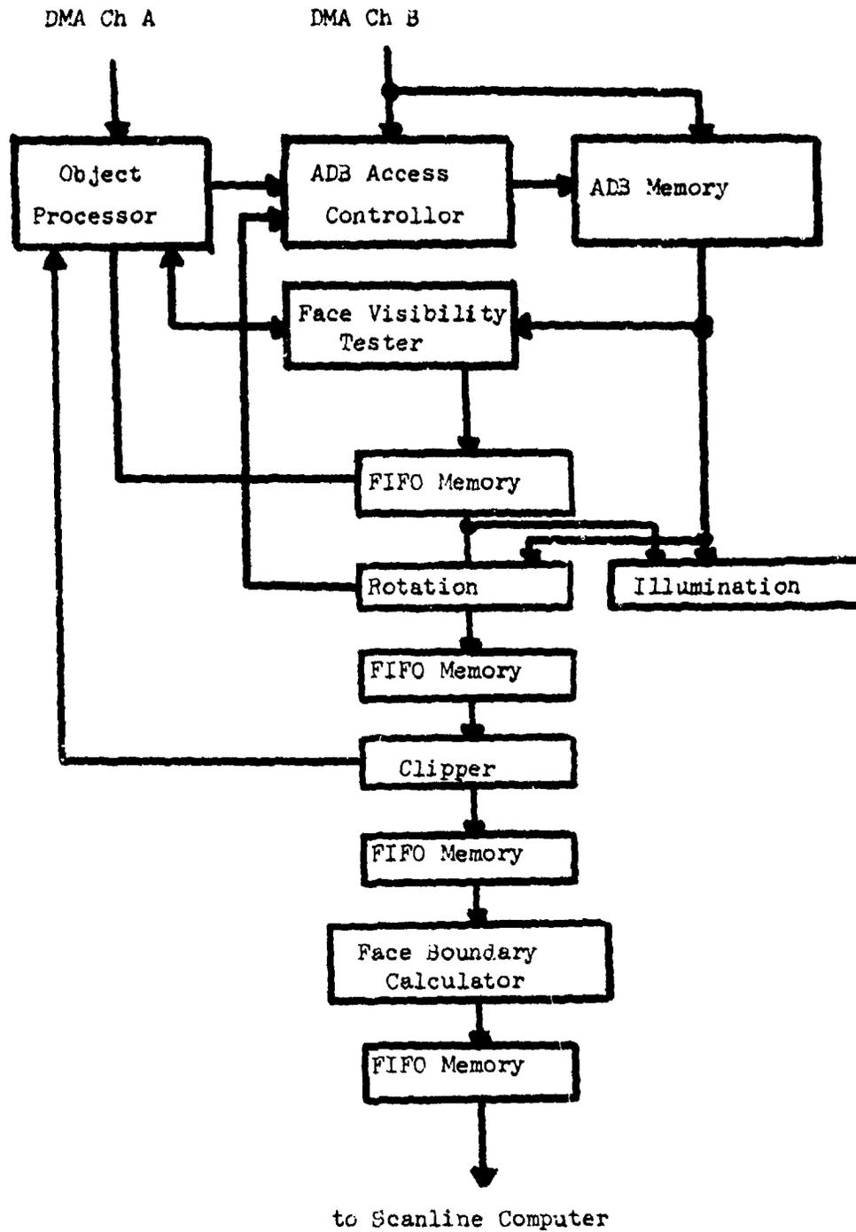
Figure 2.2.1.2.1-5. Frame Calculator Block Diagram
