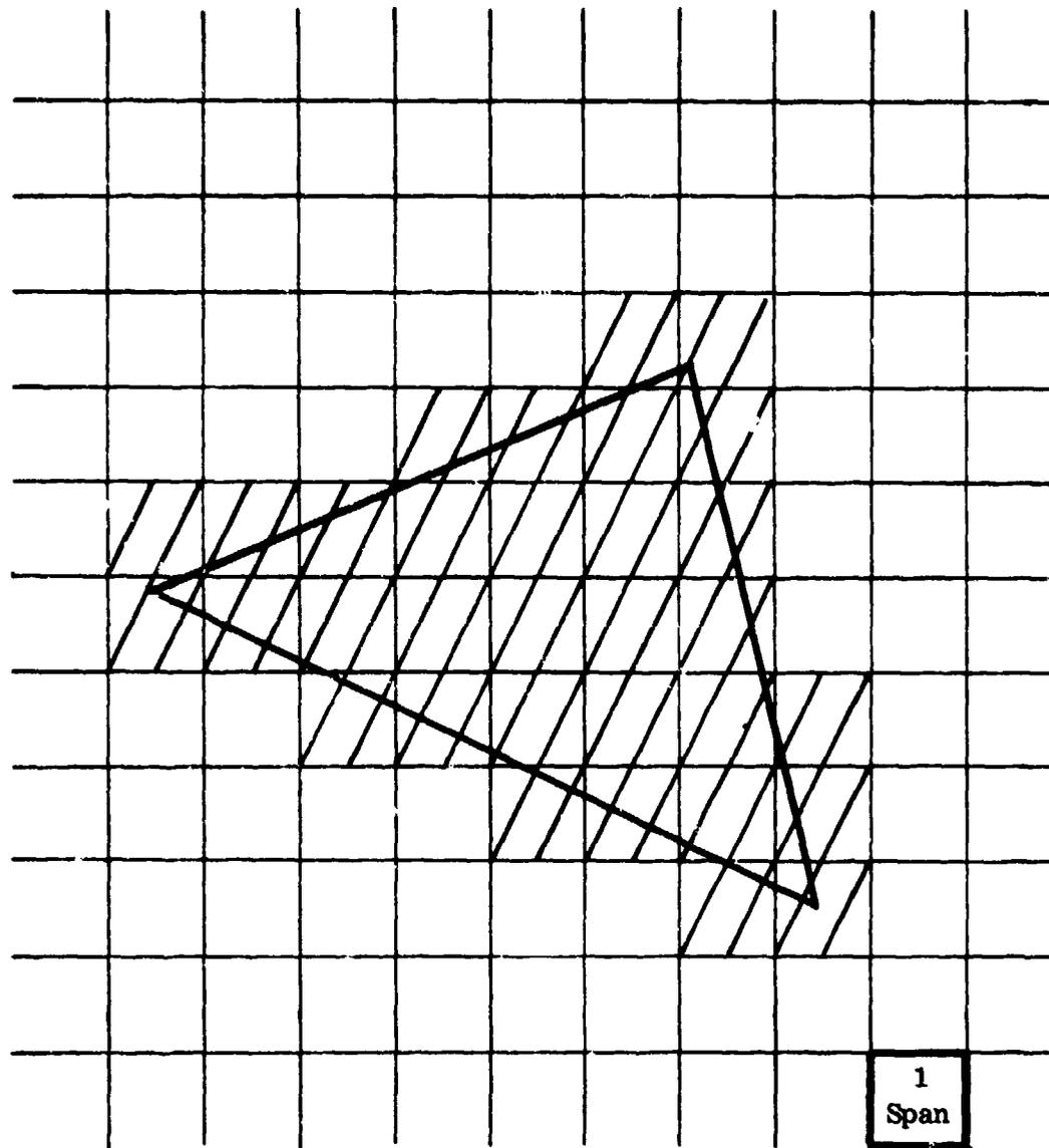
Figure 2.2.1.2.7-2. Dissection of a Polygon into Spans
