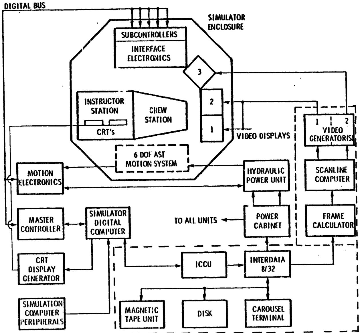
Figure 2.2.1.2.1-1. Singer Link Flight Simulator System Diagram
