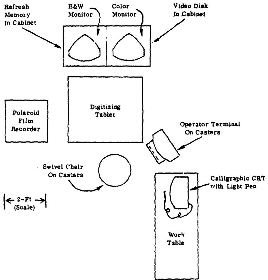
Figure 4.4.1-2. Floor Plan of Typical Graphic Work Station
