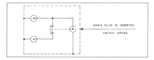
As the connector used at the terminal end is truly coaxial rather than the previously used contact finger-wiper arrangement, the system now insures long life and a constant impedance match. The maximum VSWR is 1.1.
