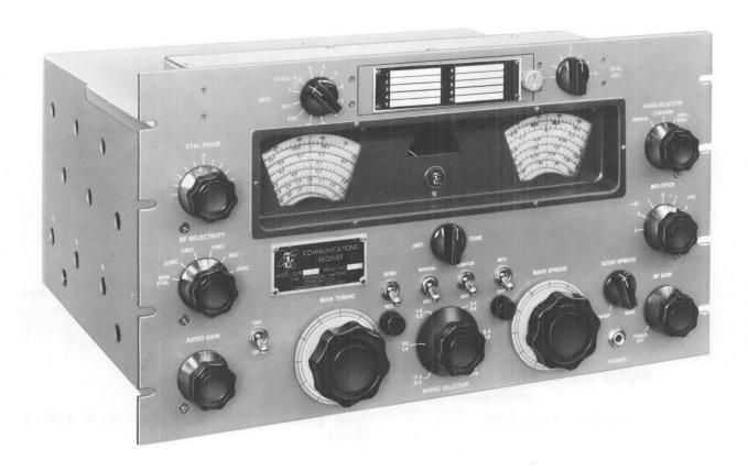
The Technical Materiel Corporation's Model GPR-91RXD Communications Receiver has all of the fine features of the widely accepted GPR-90RXD receiver *plus* 15 kc bandpass for ISB reception of four voice channels or up to 64 teletypewriter channels, when used with Model SBC-2 (AN/URA-42/TD-410/UGC) sideband converter.
