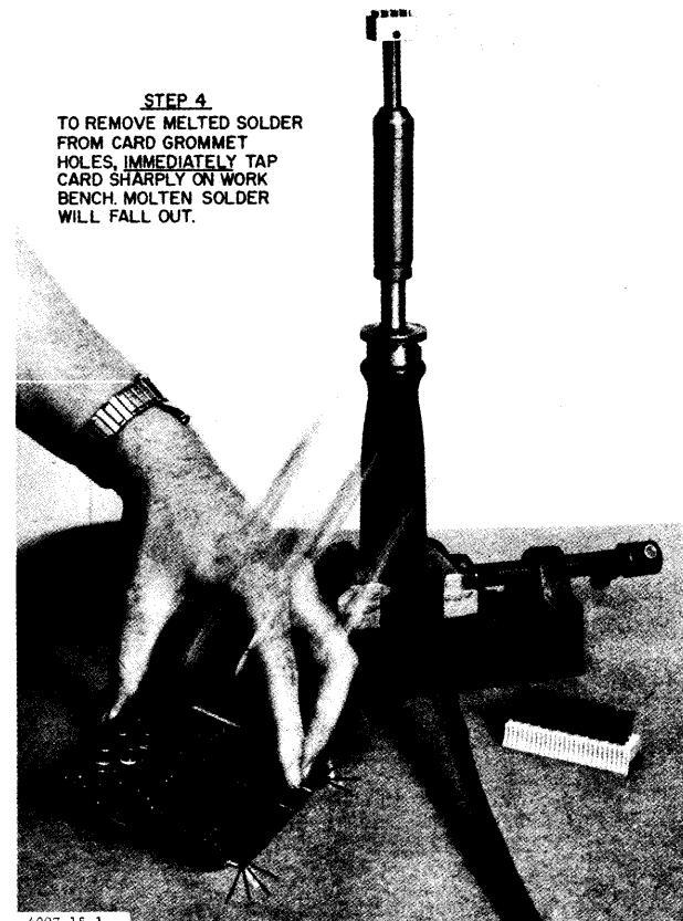
Figure 5-17. Removing Logic Module from Card
