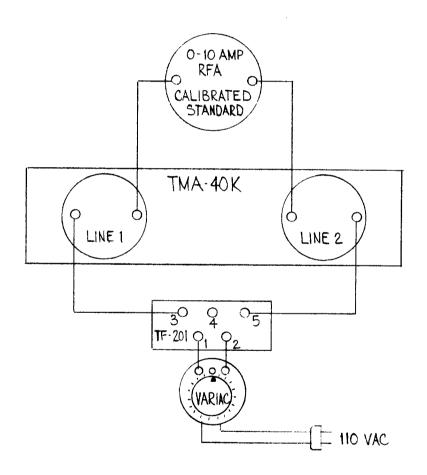
II. Procedure: Check meters for Zero adjust and before plugging into 110 VAC outlet, set variac to ZERO. By adjusting the variac for a 5 amp and 10 amp deflection on the calibrated standard, the Line 1 and Line 2 meters, when compared with the calibrated standard, should read within 5% of the full scale value. Record Line 1 and Line 2 meter readings on test data sheet.
