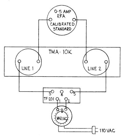
II. Procedure: Check meters for Zero adjust and before plugging into 110 VAC outlet, set variac to ZERO. By adjusting the variac for a 3 amp and 5 amp deflection on the calibrated standard, the Line 1 and Line 2 meters, when compared with the calibrated standard, should read within 5% of the full scale value. Record Line 1 and Line 2 meter readings on test data sheet.
