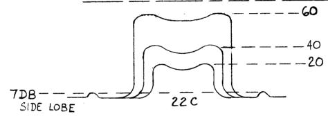
D. When the Log Amp. is overloaded, the following illustration (22D) will appear.
