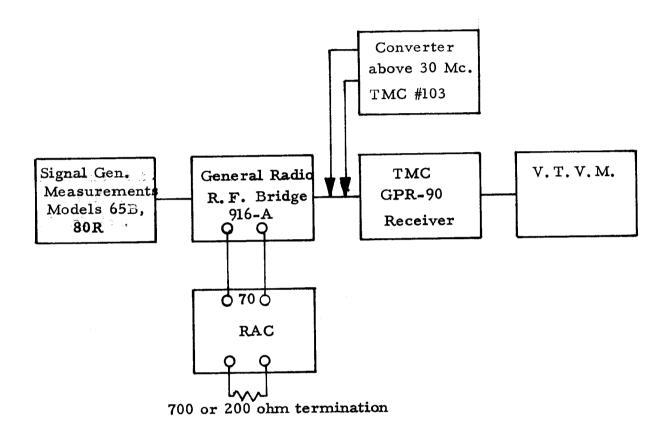
Resistance and Reactance measurements are made in accordance with the instructions supplied by the General Radio Company.
