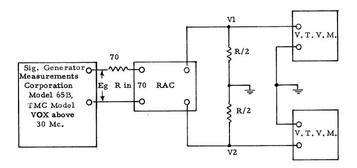
R/2 = 350 ohms for 700 ohm termination R/2 = 100 ohms for 200 ohm termination
