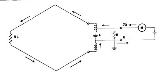
A simplified diagram is shown above showing capacitor function in DC measurements.
