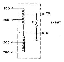
The resistor R across the  $70\Omega$  input has a value of 10K ±20% and since 10K >> 70 its shunting effect on the  $70\Omega$  winding is negligible. The purpose of this resistor is to allow a leakage path to ground for static charges which may accumulate on the antenna.
