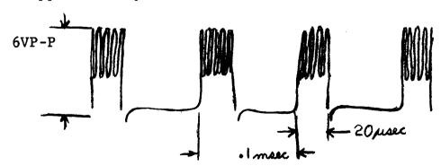
Connect a low capacity scope probe between the 3. junction of L5 and R21 and ground. Peak C11 for maximum level. The 6.29 mcs. signal displayed should be at approximately 10VP-P.
