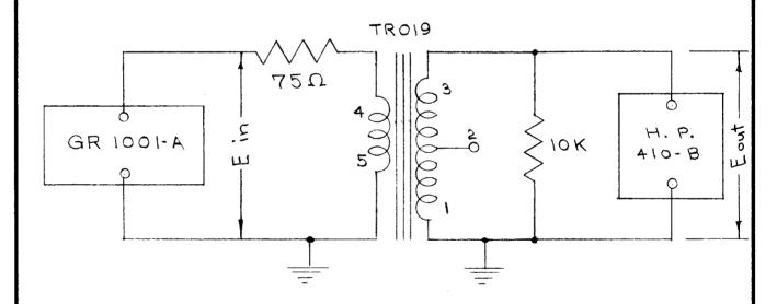
Output Voltage --- at 50 KC and 200 KC must be greater than 7.5 v lts.
