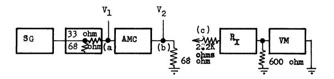
The 2.2K ohm resistor is to prevent any serious change in the AMC termination when the detector is connected.
