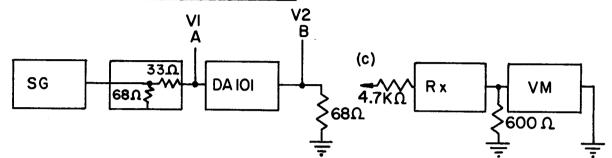
The 4.7 K ohm resistor is to prevent any serious change in the DA-101 termination when the detector is connected.
