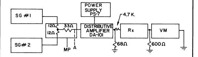
(a) Inject two signals with a level of 250 mV each, measured at the input jack - (point A)
