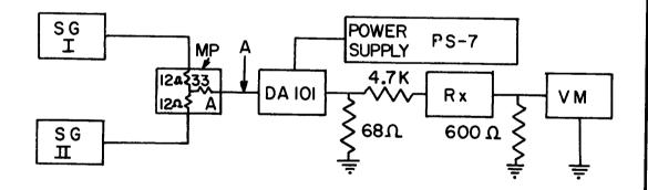
Inject two signals with a level of 250 mV each measured at the input jack J201 of the DA-101 (point A):
