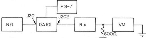
Follow the standard procedure for noise measurement. (In accordance with Proceedings of IRE July 1953, paras. 10.1.2.2, 10.1.2.2.1, 10.1.4) The following table gives the maximum readings of the meter indication:
