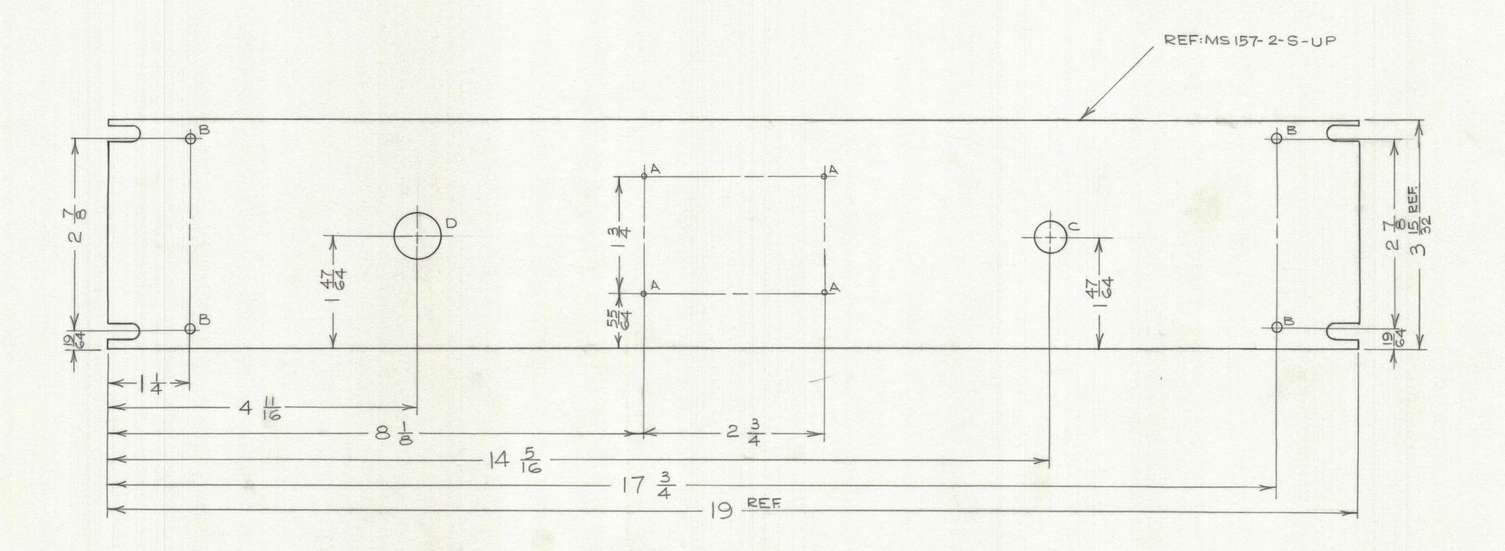
HOLE A - NO. 47 DRILL. HOLE B - 9/64 DIA. HOLE C - 1/2 DIA. HOLE D - 11/16 DIA.
