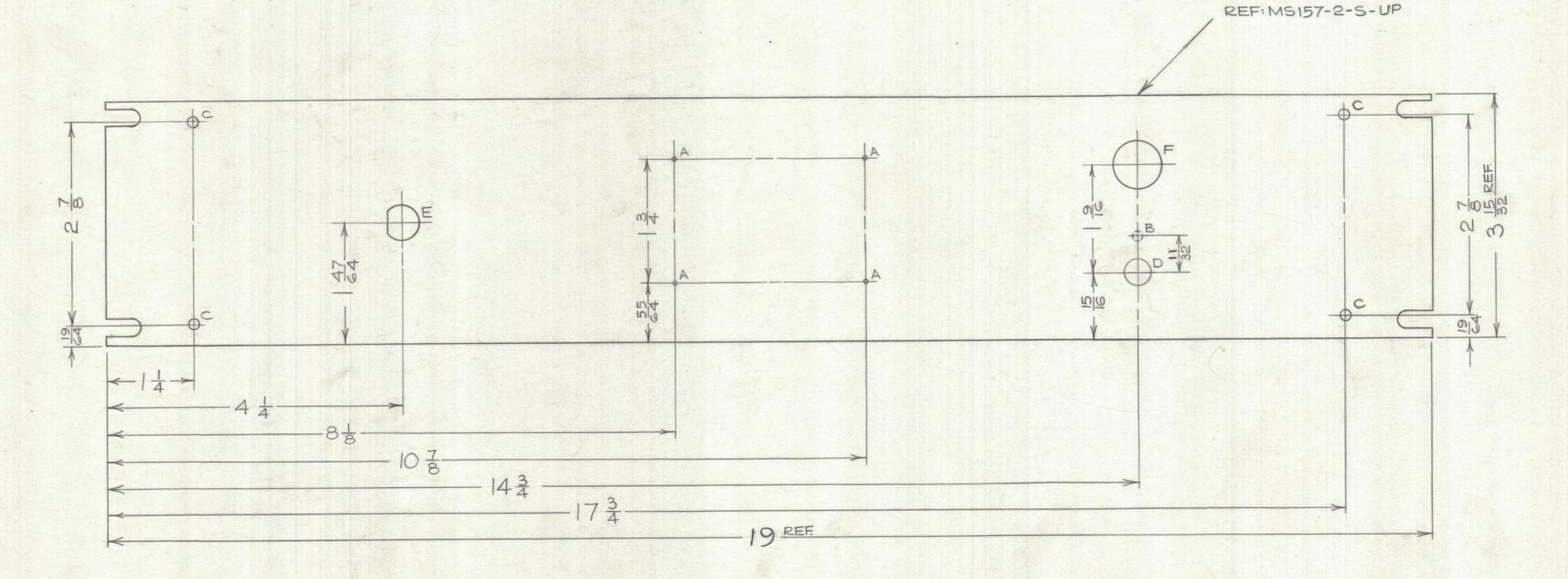
HOLE A - No. 47 DRILL. - 4 REQ HOLE B - 9/64 DIA., I/8 DEEP FROM REAR OF PANEL - 1 REQ HOLE C - 9/64 DIA. - 4 REQ HOLE D - 1/4 DIA. - 1 REQ HOLE E - 1/2 DIA., D."-1 REQ HOLE F - 11/16 DIA. - 1 REQ
