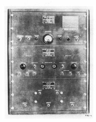
Frequency Shift Receiver Equipment FRC-1 is used to demodulate frequency-shift-keyed radioteletype signals by converting a-f signals to polar-keyed teletypewriter impulses. It functions at audio frequencies and therefore may be used with any stable communication receiver equipped with a beat-frequency oscillator.
