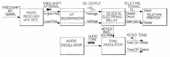
Figure 2-1. Simplified Block Diagram
