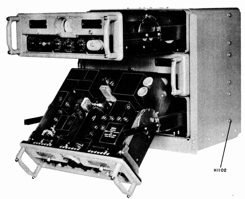
Figure 1-2. View of Drawer Slides and Tilt Action in Units of AN/URA-8A Equipment
