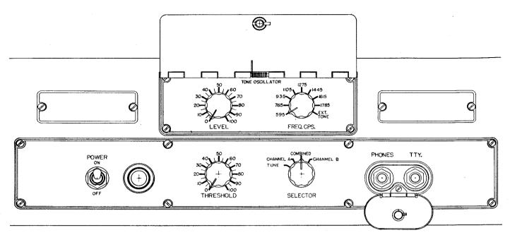
Figure 4-2. Comparator CM-22/URA-8A, Operating Controls
