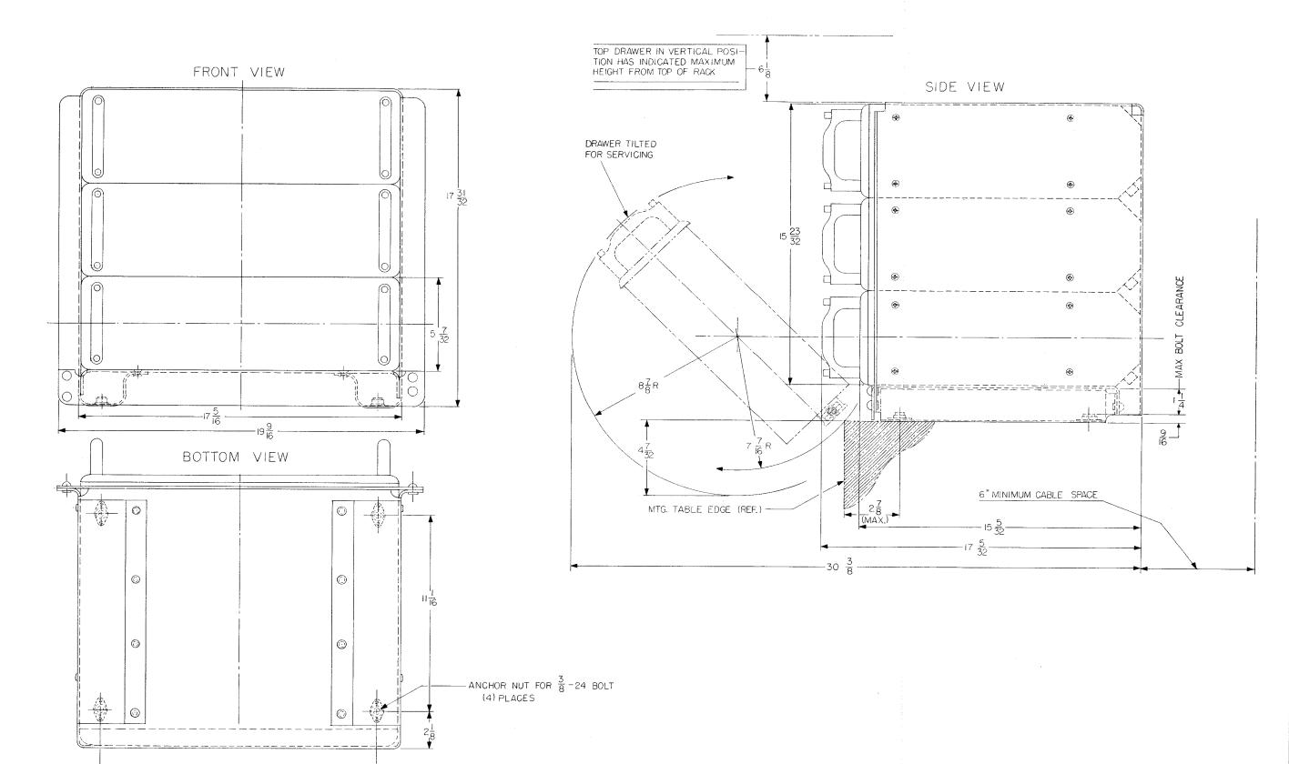
Figure 3-6. Frequency Shift Converter-Comparator Group AN/URA-8A, Installation Drawing
