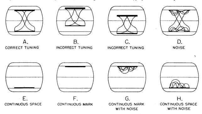
Figure 4-3. Monitor Oscilloscope Patterns
