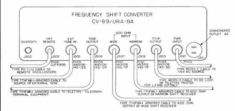
Figure 3-5. Interconnecting Cable Diagram, Single Receiver Operation
