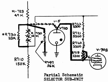
\*NOTE: If Field Change #1 which converts R-730 from 33K ohms to 10K ohms has not been accomplished the revision of this resistor to 33K ohms is not applicable.
