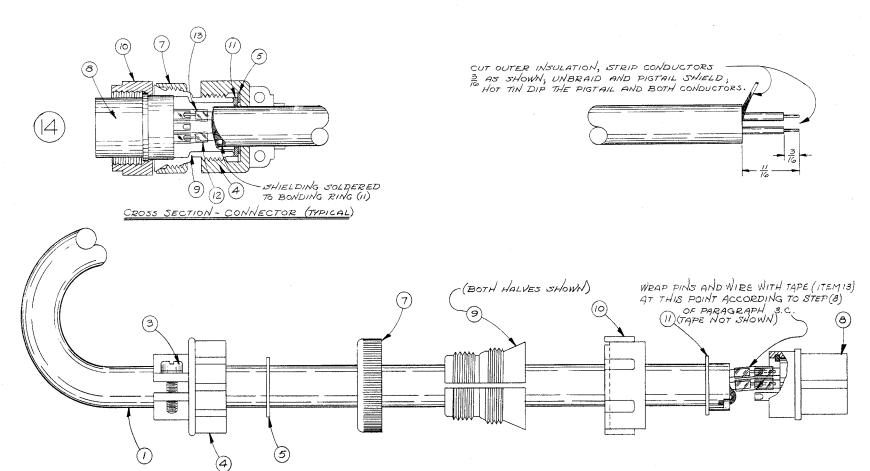
TABLE 3-1. TERMINATIONS FOR MCOS-2 CABLE USED FOR EXTERNAL CONNECTIONS
