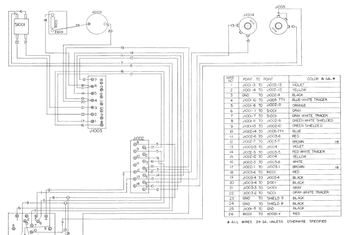
Figure 5-28. Comparator Chassis-Panel Assembly, Wiring Diagram
