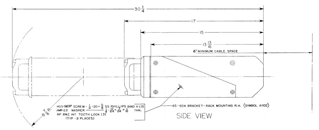
Figure 3-8. Rackmounted Unit, Installation Drawing
