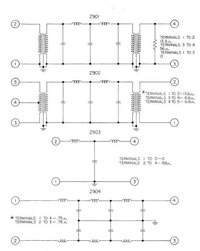
\* FOR FILTERS MARKED WITH AN ASTERISK, THE INSULATION RESISTANCE BE-TWEEN ANY TERMINAL AND CASE WILL NORMALLY BE 50 MEGOHMS OR HIGHER WHEN MEASURED WITH A POTENTIAL OF 500 VOLTS.
