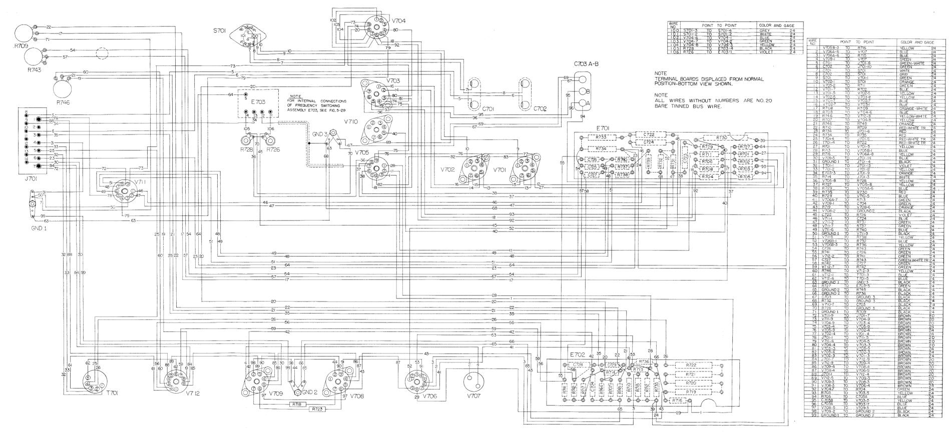
Figure 5-25. Selector Sub-Unit, Wiring Diagram
