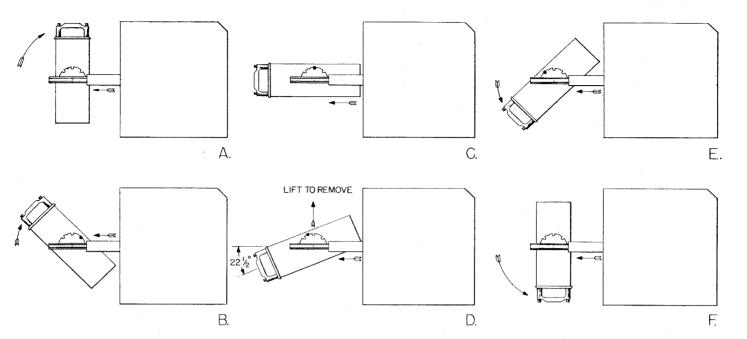
Figure 5-2. Tilt Positions of Drawer Assembly
