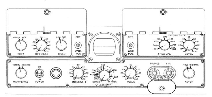
Figure 4-1. Frequency Shift Converter CV-89/URA-8A, Operating Controls
