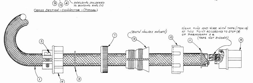
CUT OUTER INSULATION, STRIP CONDUCTORS 3 AS SHOWN, UNBRAID AND PIGTAIL SHIELD, IN HOT TIN DIP THE PIGTAIL AND BOTH CONDUCTORS.
