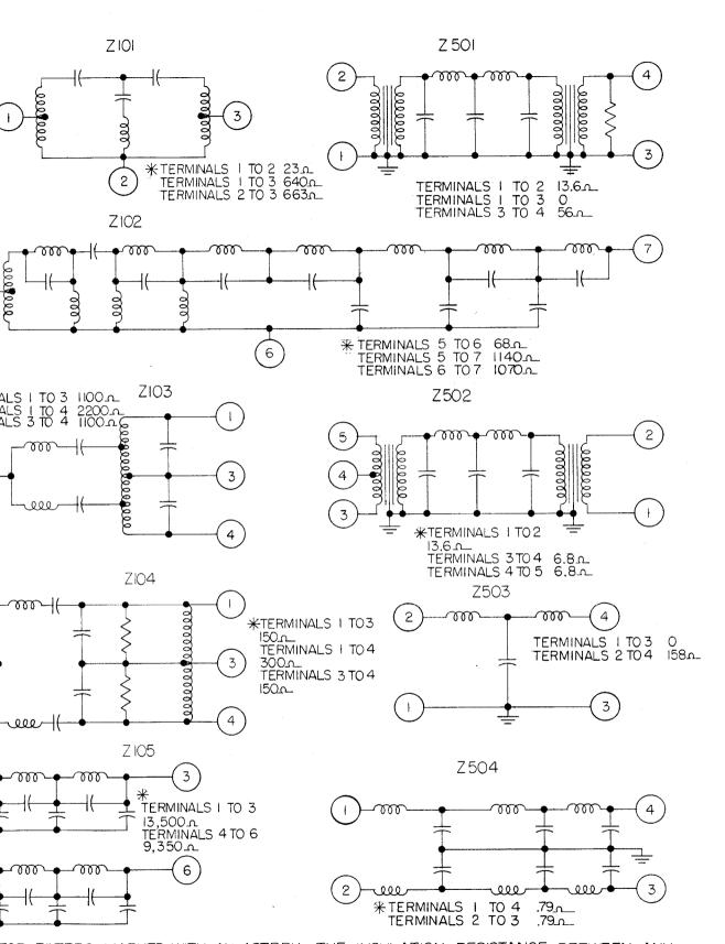
FOR FILTERS MARKED WITH AN ASTERK, THE INSULATION RESISTANCE BETWEEN ANY TERMINAL AND CASE WILL NORMALLY BE 50 MEGOHMS OR HIGHER WHEN MEASURED WITH A POTENTIAL OF 500 VOLTS.
