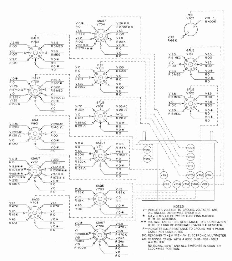
Figure 5-4. Comparator Voltage and Resistance Chart
