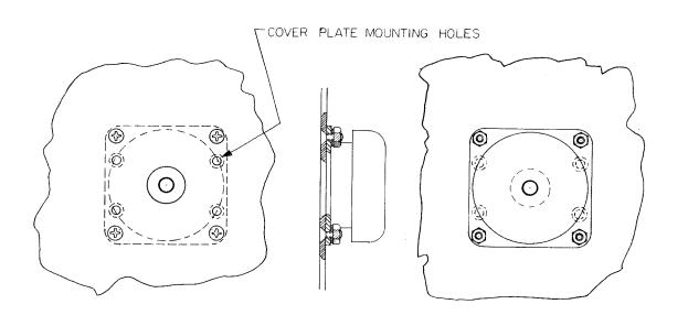
DETAIL OF SHOCKMOUNTS HG-20 (SYMBOL A603) FASTENING USE SCREWS, WASHERS & NUTS THAT HOLD HOLE COVER PLATE (AS-443 IN POSITION.
