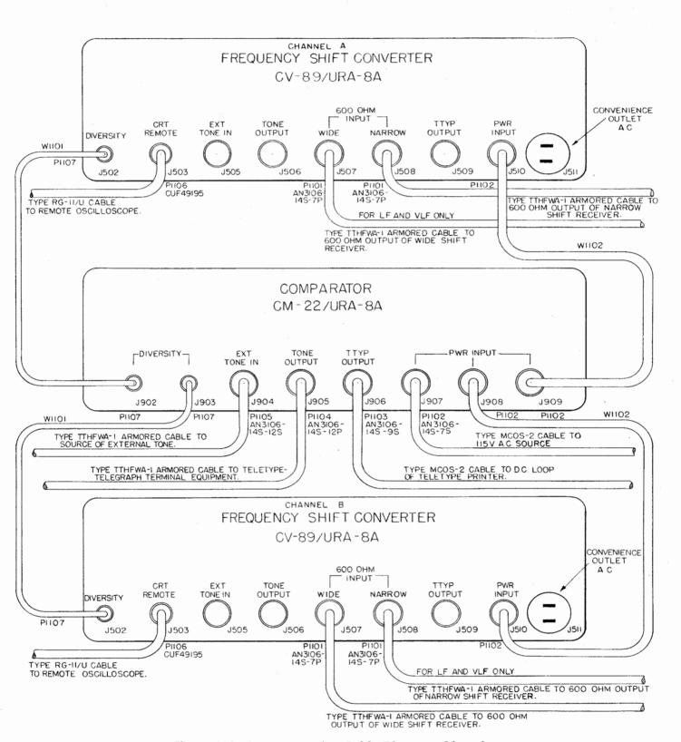
Figure 3-1. Interconnecting Cable Diagram, Diversity
