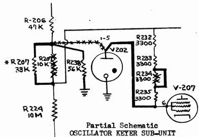
\*NOTE: If Field Change #1 which converts R-207 from 33K ohms to 10K ohms has not been accomplished the revision of this resistor to 33K ohms is not applicable.
