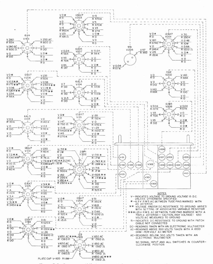
Figure 5-3. Frequency Shift Converter Voltage and Resistance Chart
