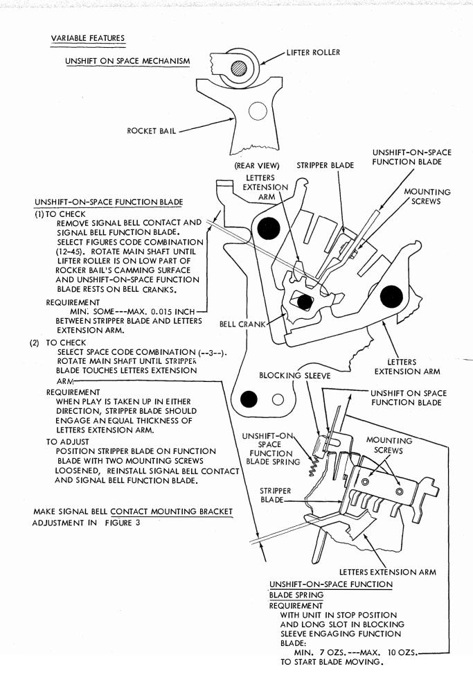
FIGURE 2. UNSHIFT ON SPACE MECHANISM
