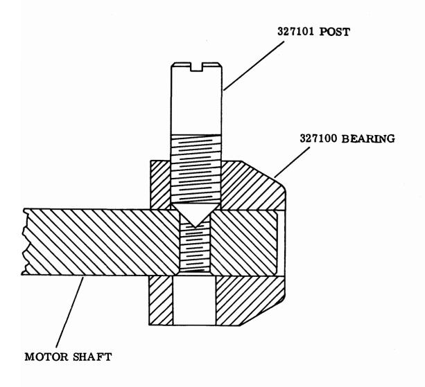
NOTE: POINT OF POST TO SEAT IN TAPPED HOLE OF MOTOR SHAFT
