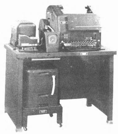
TELETYPE MODEL 19 SET WITH MODEL 14 REPERFORATOR
