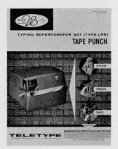
LPR—Model 28 Typing Reperforator Set, 5 level code, printed "chadless" tape, optional gear shift for changing to slower speeds.
