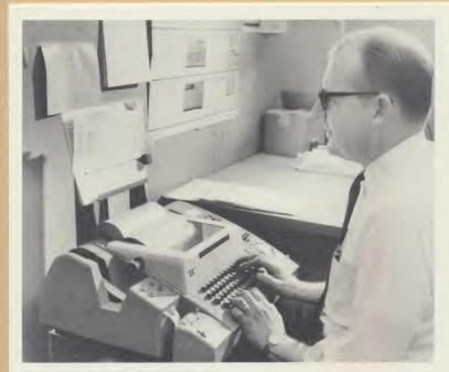
Engineers and scientists at Appliance Park communicate directly with the computer via a Teletype Model 33 ASR (automatic send-receive) set. The "conversation" is recorded as page copy, but a paper tape can be punched simultaneously. Shown here is Stuart R. Kunz, Specialist Engineering, Merchandized Information Systems.
