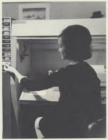
Each computer program developed at the Applied Mathematics Laboratory is punched into paper tape by the operator of a Teletype Model 35 ASR (automatic send-receive) set, as demonstrated by Mrs. Betty Hall, computer programmer. Tapes are then stored until an engineer or scientist has application for a particular one, at which time the tape is inserted into the ASR set's tape reader and transmitted to the computer.
