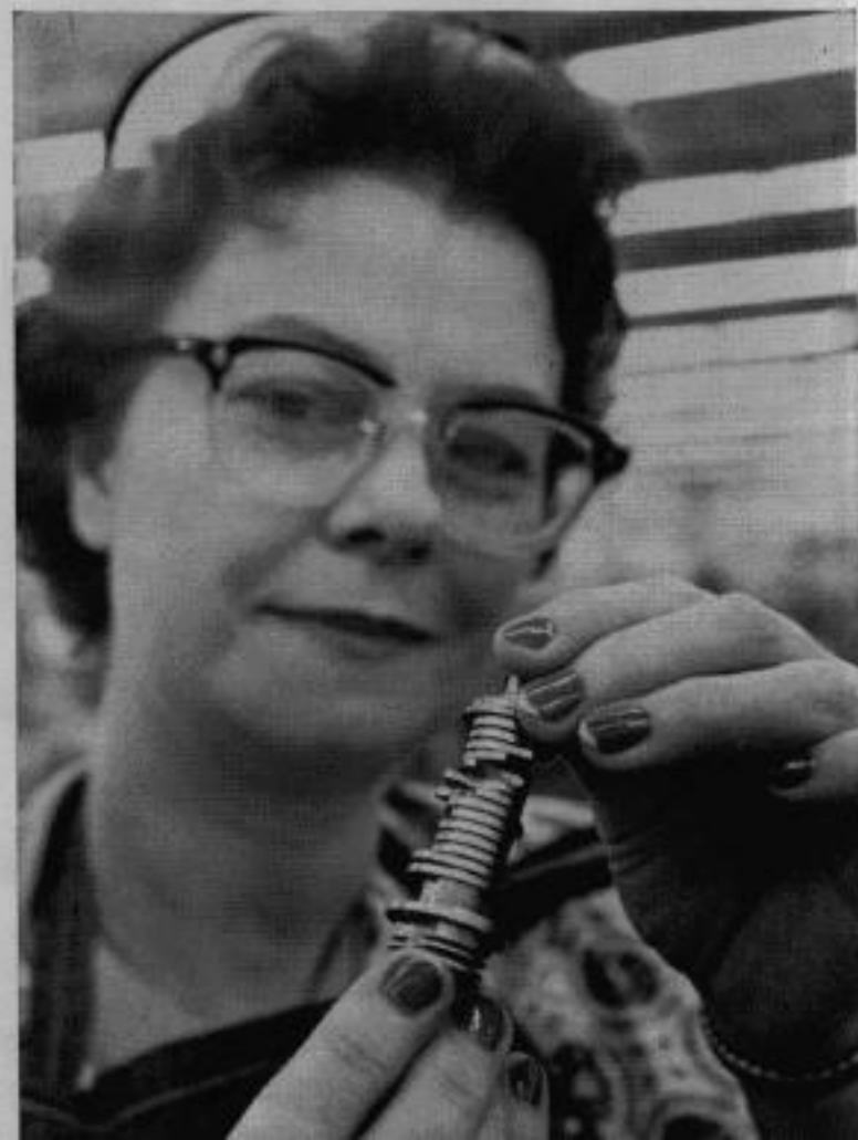
INSIDE STORY. Internal mechanisms of Model 28 teletypewriters get final adjustment at new Teletype plant. Below, Ann McGregor displays close-tolerance timing cam, key part of '28' series.
