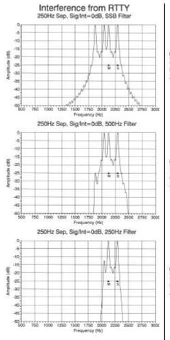
Figure 7. Interference, 250 Hz Spacing, Equal Amplitude
