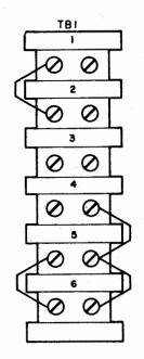
Figure 2-2. Terminal Board Connection 48-Volt Output
