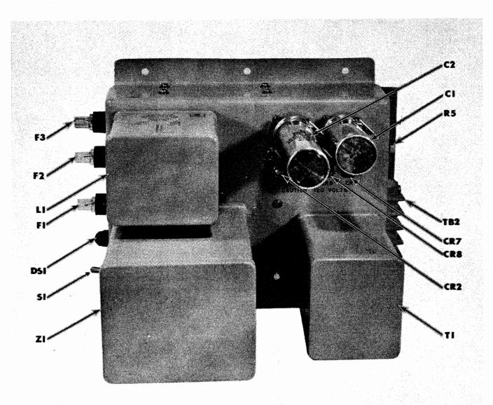
Figure 6-1. Power Supply PP-3495/UG, Top View
