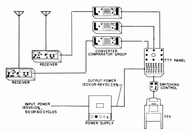
Figure 1-2. Power Supply PP-3495/UG, System Diagram
