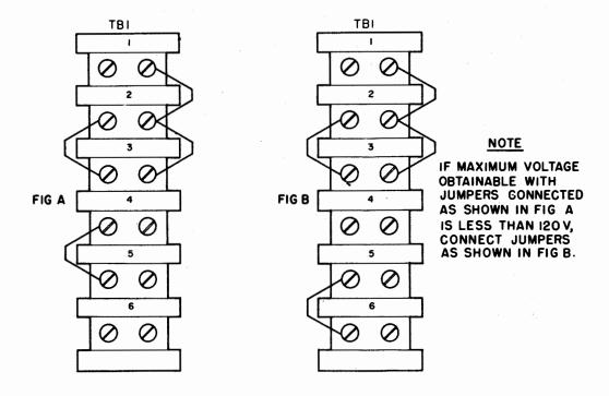
Figure 2-3. Terminal Board Connections 120-Volt Output
