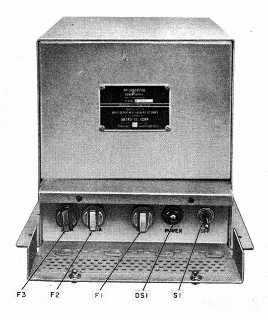
Figure 3-2. Power Supply PP-3495B/UG, Front View
