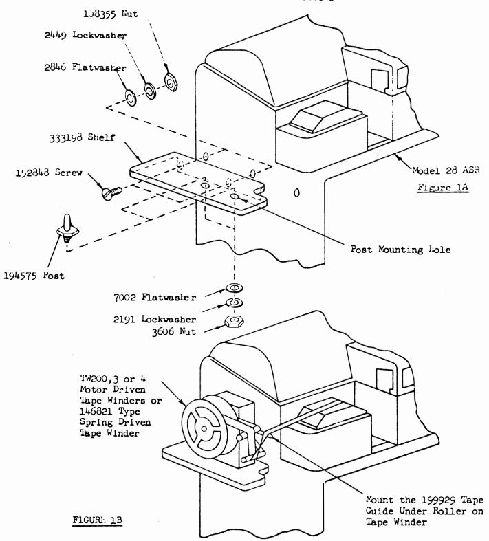
321582 Modification Kit: To Provide Mounting Shelf for Single Reel Tape Winder on Upper Left Side of Model 28 ASR
