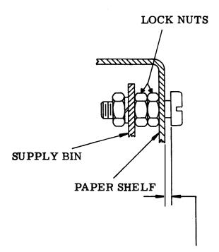
Requirement: The Accumulating Shelf Should Pivot Freely on The Supply Bin. There Should Be Approximately 1/64 Inch Clearance.
