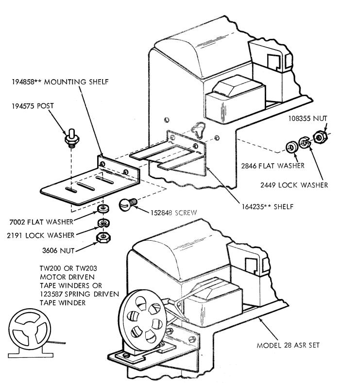
194857\*\* MODIFICATION KIT: TO PROVIDE MOUNTING SHELF ON THE LEFT SIDE OF THE ASR SET FOR THE SINGLE REEL TAPE WINDER
