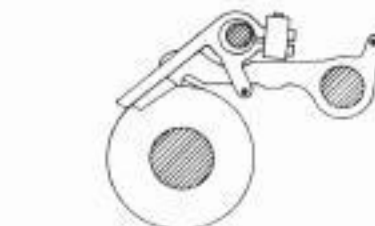
Figure 5-31. Clutch Back-Stop Adjustment
