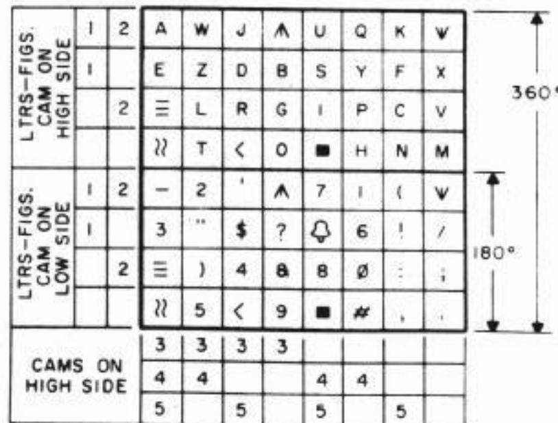
Figure 5-64. Plan View of Print Cylinder
