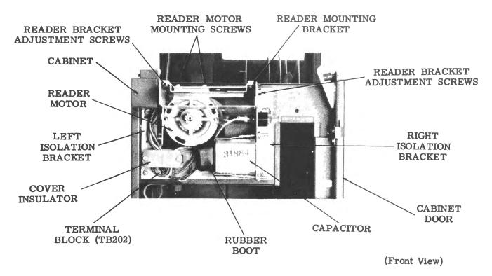
Figure 20 - Reader Motor Removal
