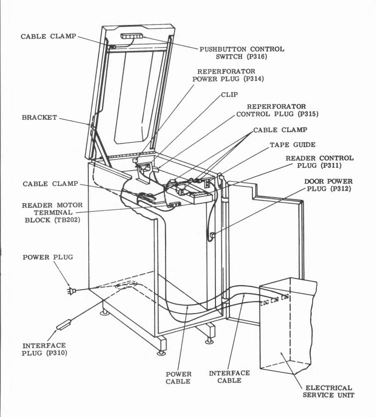
Figure 22 - Tape Module Cable Routing
