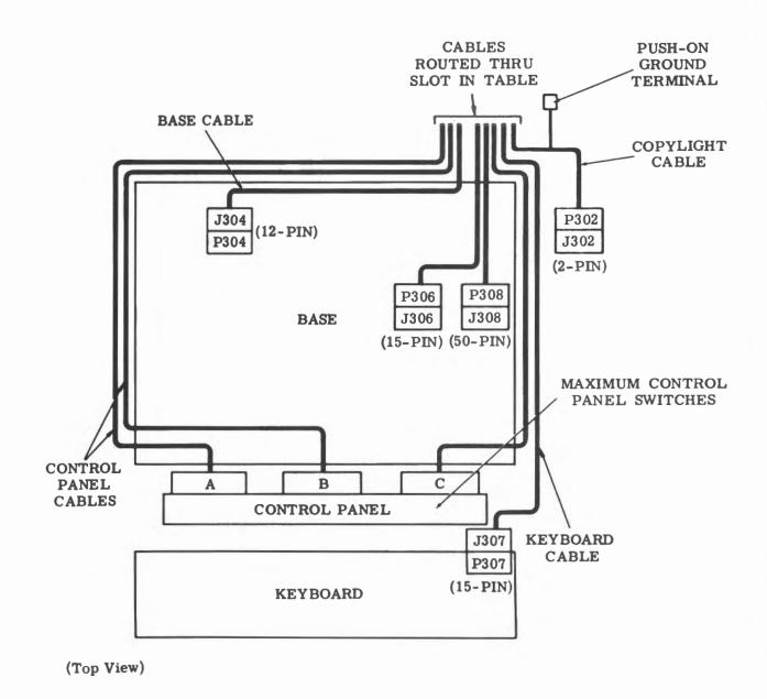
Figure 11 - Cable Routing Above Table
