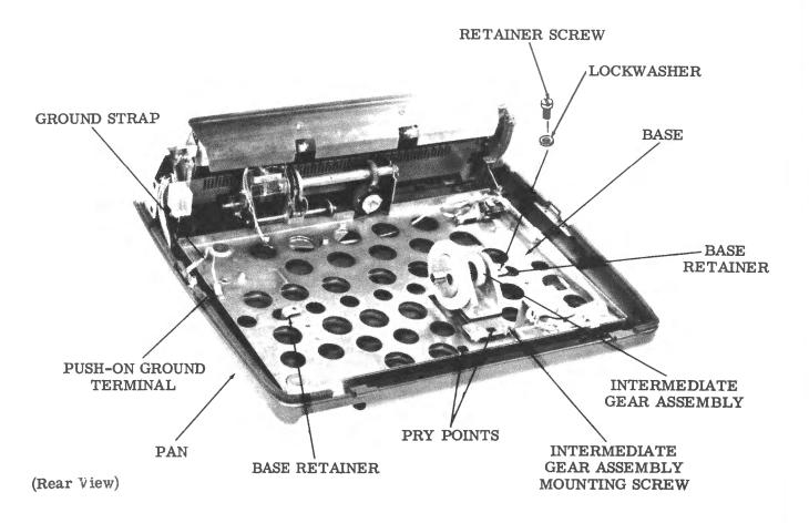
Figure 8 - Keyboard, Control Unit, Reset Mechanism, and Intermediate Gear Assembly
