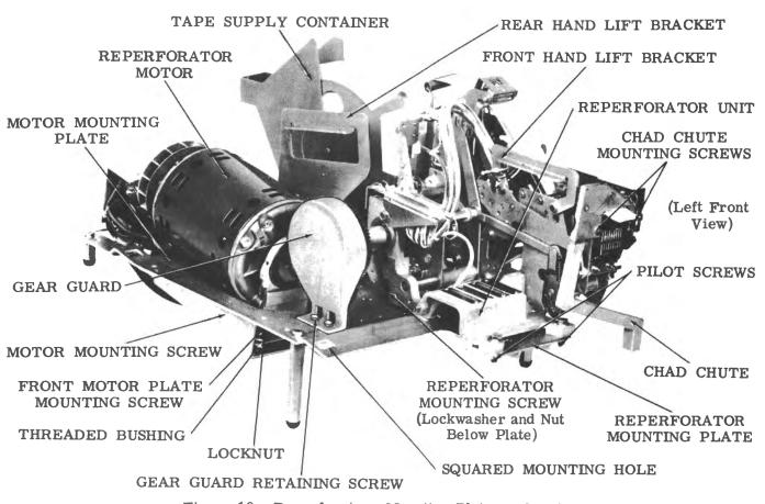
Figure 18 - Reperforator, Mounting Plate, and Motor
