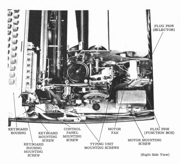
Figure 3 - Typing Unit and Control Panel
