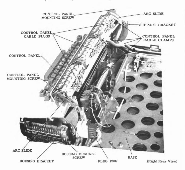
Figure 6 - Control Panel and Keyboard
