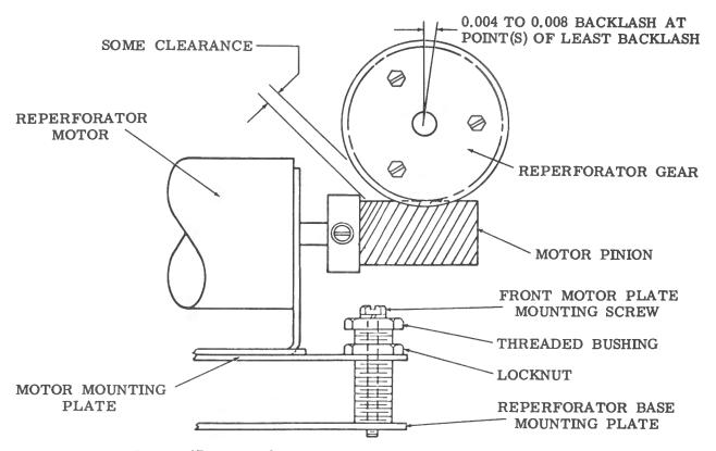
Figure 17 - Reperforator Motor Pinion and Gear Mesh
