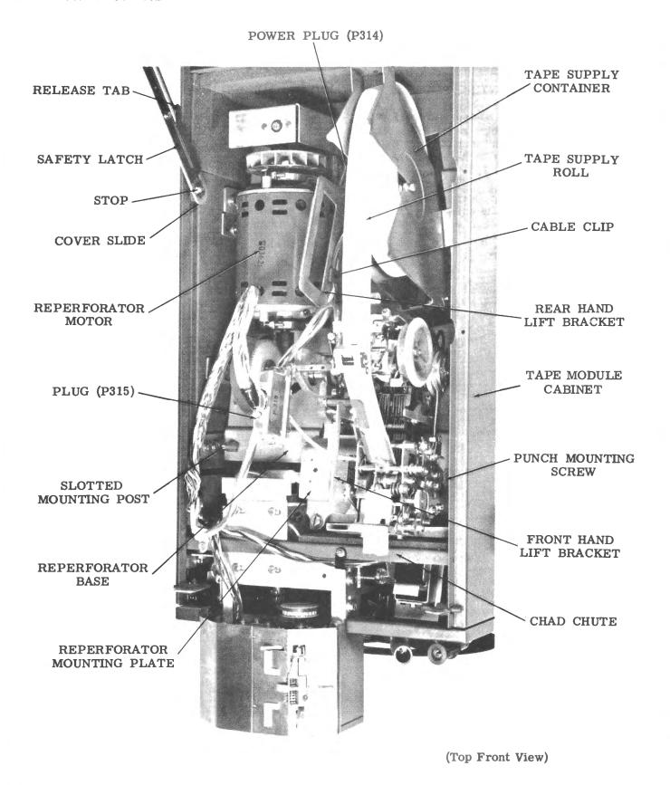
Figure 16 - Tape Module (Cabinet Opened)
