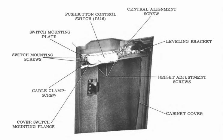
Figure 21 - Pushbutton Switch Removal
