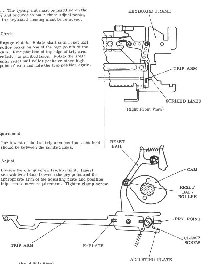
Figure 5 - Keyboard Trip Arm Adjustment
