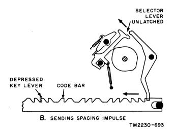
Figure 37. Operation of transmitting mechanism.
