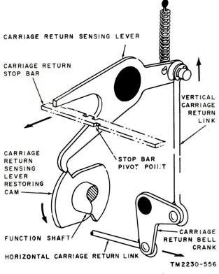
Figure 53. Carriage return operating mechanism as seen from the rear of the teleprinter.
