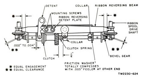
Figure 227. Ribbon spool drive shaft and clutch spring adjustments.
