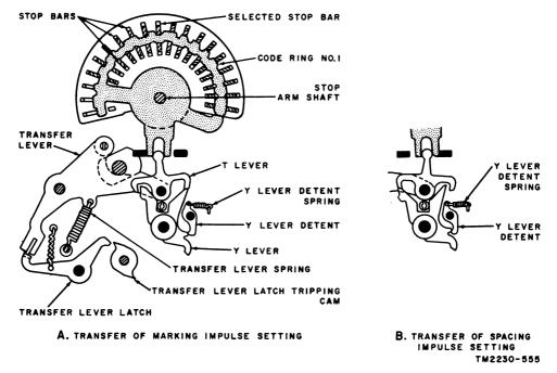
Figure 42. Transfer mechanism operation.
