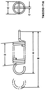
Figure 248. Parallel-end spring.
