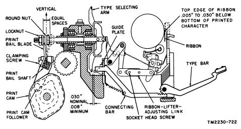
Figure 224. Printing bail and ribbon lifter adjustments.
