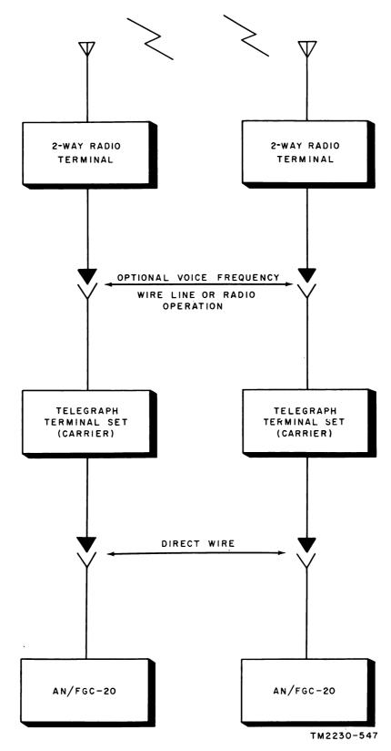
Figure 3. Carrier, direct wire, or radio system, block diagram.
