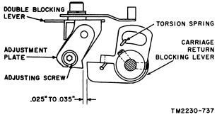
Figure 199. Carriage return adjustment plate adjustment.
