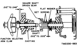
Figure 158. Square shaft driven gear adjustment.
