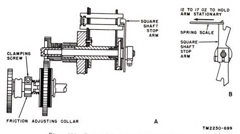
Figure 184. Square shaft stop arm torque adjustments.
