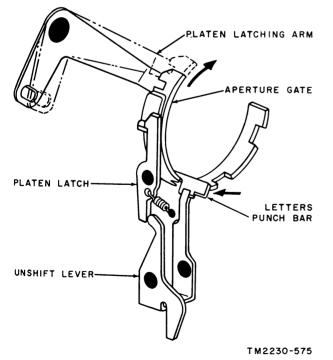
Figure 64. Aperture gate latched.
