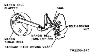
Figure 233. Margin signal bell adjustment.
