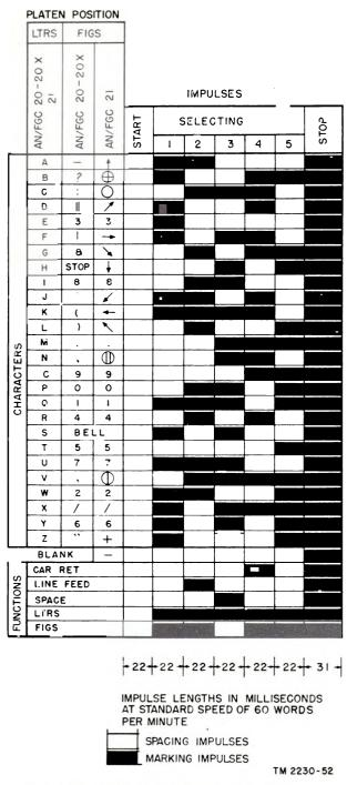
Figure 26. Standard start-stop, five-unit code chart.
