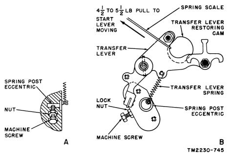
Figure 182. Transfer lever spring adjustment.
