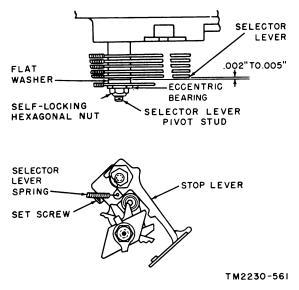
Figure 152. Selector lever clearance adjustment.
