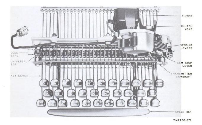
Figure 34. Keyboard transmitter parts.
