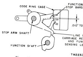
Figure 161. Code ring cage adjustment.
