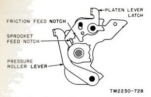
Figure 208. Pressure roller lever position adjustment.
