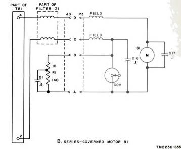
Figure 86. Motor and copy lamp circuits, simplified schematic.
