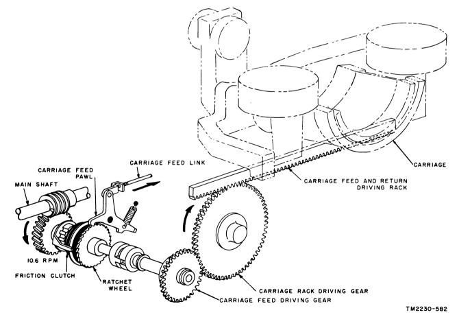
Figure 55. Carriage feed mechanism.
