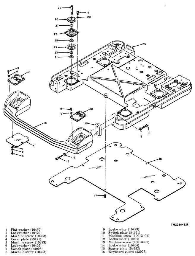
Figure 146. Teleprinter base and keyboard guard, exploded view.
