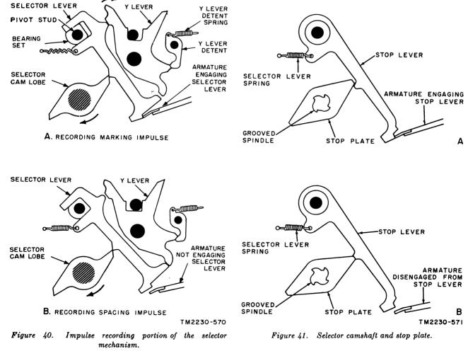
by the subsequent positioning of the selector mechanism of the teleprinter.
