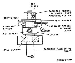
Figure 197. Carriage return blocking lever clearance adjustment.
