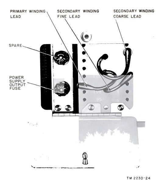
Figure 12. Power supply fuse and leads.
