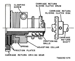
Figure 60. Can iage veturn safety clutch.
