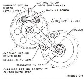
Figure 189. Carriage return tripping arm adjustment.
