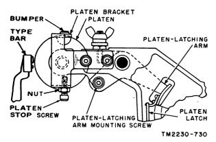
Figure 214. Letters shift position adjustment.
