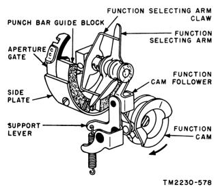
Figure 51. Function selecting arm mechanism.
