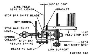
Figure 231. Automatic carriage return, stop bar shift blade adjustment.
