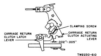
Figure 194. Carriage return clutch actuating lever adjustment.
