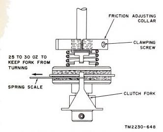
Figure 241. Transmitter friction clutch adjustment.
