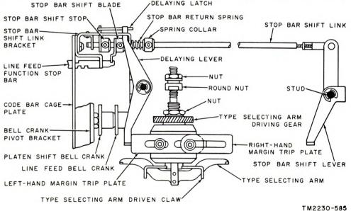
Figure 69. Automatic carriage return and line feed control.
