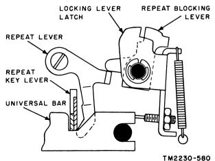
Figure 38. Repeat mechanism.
