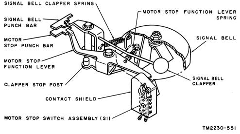
Figure 68. Signal bell and motor stop actuating mechanisms.
