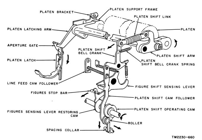
Figure 63. Figures shift mechanism.
