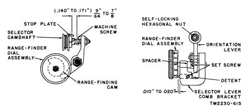
Figure 153. Rangefinder dial assembly.
