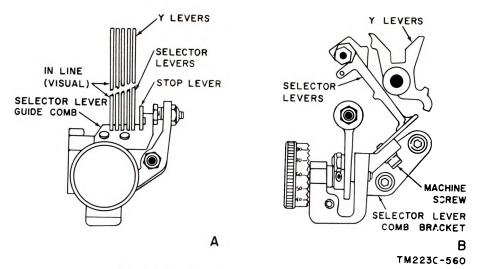
Figure 154. Selector lever guide comb adjustment.
