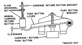
Figure 245. Manual carriage return pushbutton adjustment.
