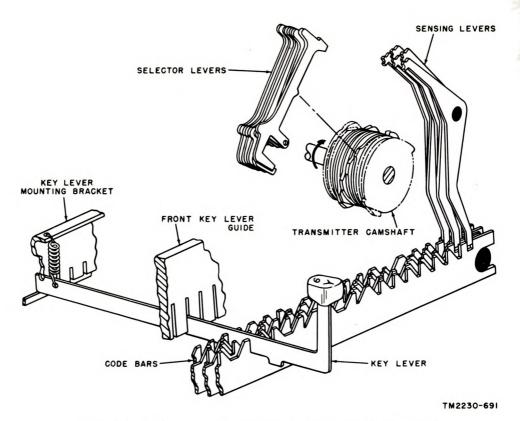
Figure 36. Setting up mechanical form of code by operating key lever.
