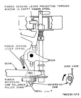
Figure 72. Inkirg ribuon reversing mechanism.
