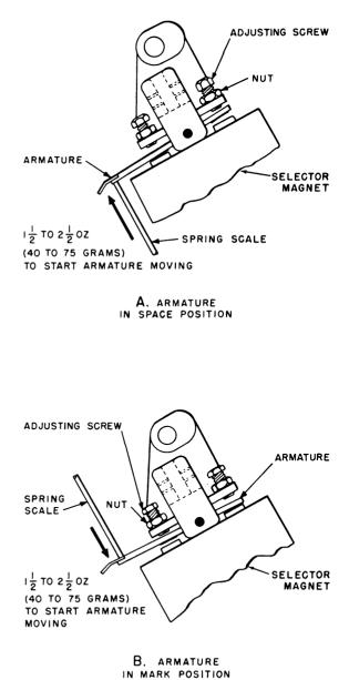
Figure 174. Magnet attractive force and armature clearance adjustment.
