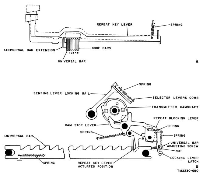
Figure 35. Transmitter camshaft control mechanism.
