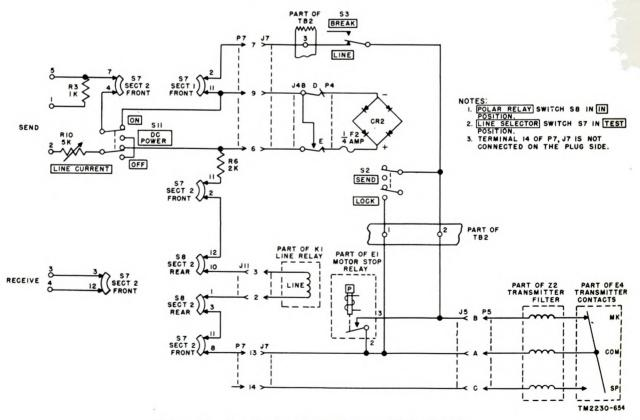
Figure 79. Test circuit with line relay, simplified schematic.
