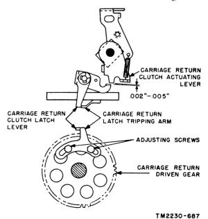
Figure 195. Carriage return clutch latch adjustment.
