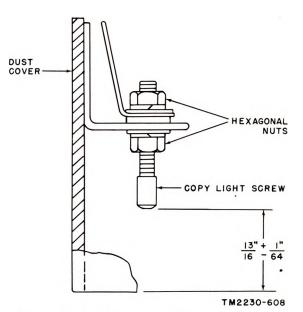
Figure 242. Dust cover copy light screws adjustment.
