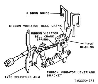
Figure 70. Inking ribbon lifter mechanism.
