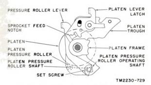
Figure 209. Platen pressure roller adjustment.
