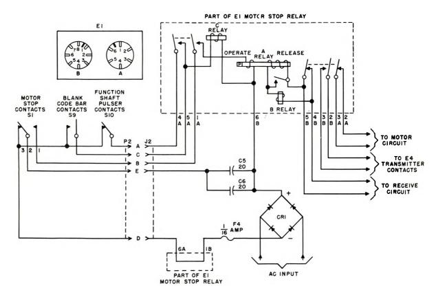
**B. TT-99/FG MOTOR STOP CIRCUIT**
