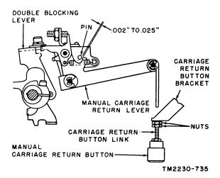
Figure 201. Manual carriage return lever adjustment.
