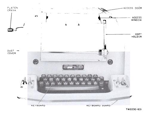
Figure 5. Teleprinter.
