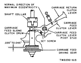
Figure 190. Carriage feed sliding clutch drum adjustment.
