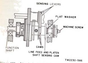
Figure 159. Line feed and platen shift sensing cam alinement.
