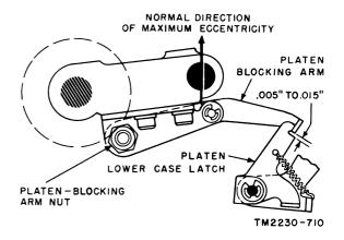
Figure 216. Platen blocking arm adjustment.
