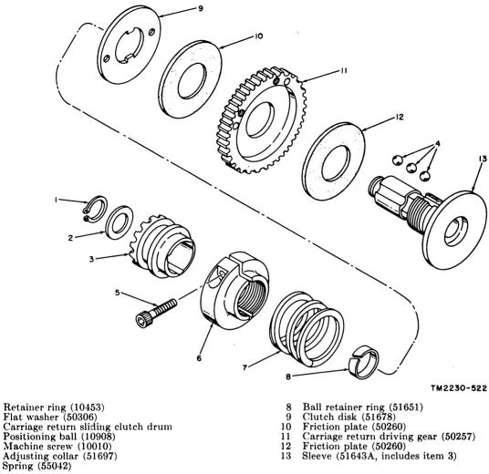
Figure 143. Carriage return safety clutch, exploded view.
