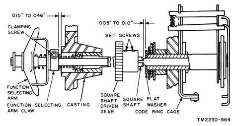
Figure 157. Square shaft and function selecting arm claw adjustment.
