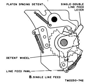
Figure 61. Single-double line feed mechanism.
