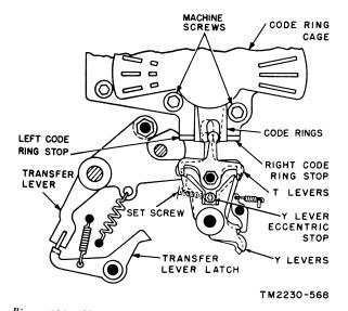
Figure 166. Y-lever eccentric stop preliminary adjustment.
