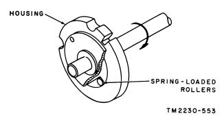
Figure 46. Antibounce clutch for stop arm.
