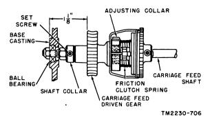
Figure 221. Carriage feed driven gear adjustment.
