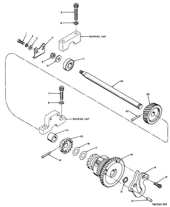
Figure 142. Carriage return shaft, exploded view.
