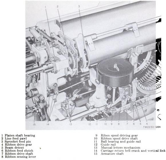
Teleprinter, left front view, showing lubrication points. Figure 95.
