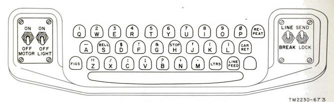
Figure 17. Standard communications keyboard.
