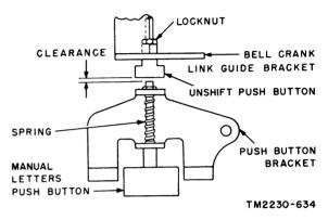
Figure 246. Manual letters pushbutton adjustment.
