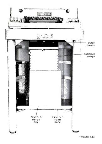
Figure 23. Fanfold paper placed in table.
