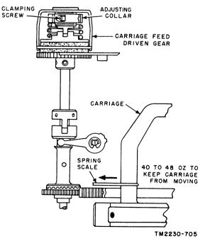
Figure 222. Carriage feed friction clutch adjustment.
