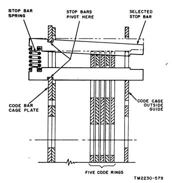
Figure 45. Code ring cage; stop bar pushed into alined code ring notches.
