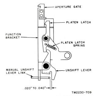
Figure 218. Manual unshift lever link adjustment.
