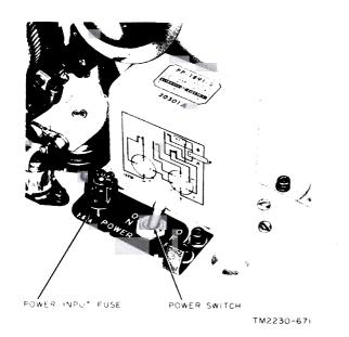
Figure 11. Power input fuse and POWER switch location.
