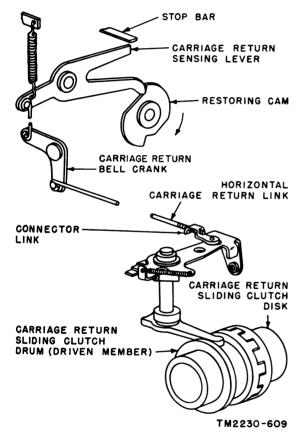
Figure 193. Carriage return clutch adjustment.
