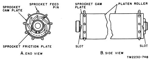
Figure 207. Sprocket feed pins, operational adjustment.
