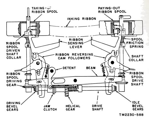
Figure 71. Ribbon feed mechanism.
