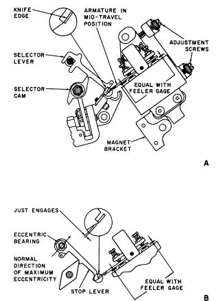
Figure 177. Selector and stop levers alinement with armature (preliminary adjustment).
