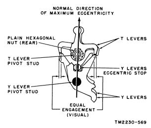
Figure 167. T-lever pivot stud adjustment.
