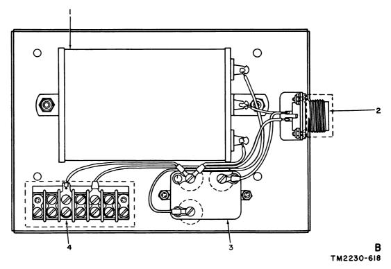
Figure 150. Motor suppression filter assembly electrical components.
