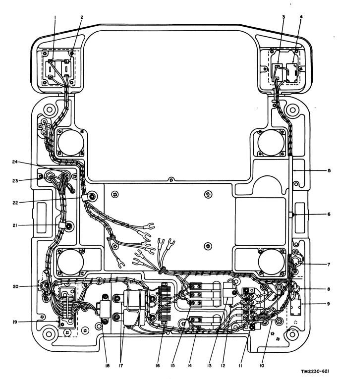
Figure 148. Teleprinter base electrical components.
