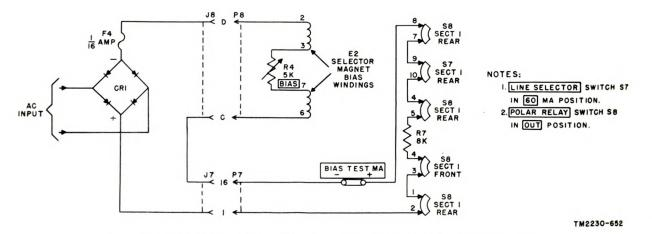
Figure 81. Selector magnet bias (60-ma) circuit, without relay, simplified schematic.
