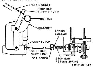
Figure 232. Automatic carriage return stop bar return spring adjustment.
