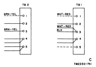
Figure 15. Wiring changes for receive only operation.
