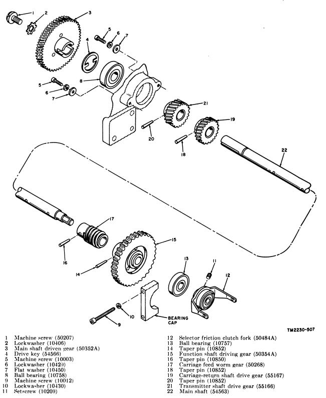
Figure 131. Teleprinter main shaft, exploded view.
