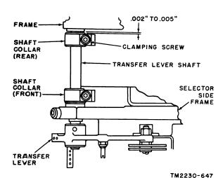
Figure 165. Transfer lever shaft end play adjustment.
