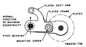
Figure 212. Platen shift preliminary adjustment.
