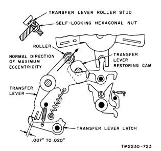
Figure 163. Transfer lever roller stud adjustment.
