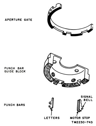
Figure 52. Punch bar guide block, aperture gate, and function punch bars.
