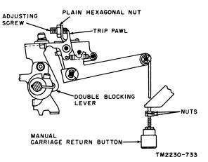
Figure 200. Manual carriage return trip pawl adjustment.
