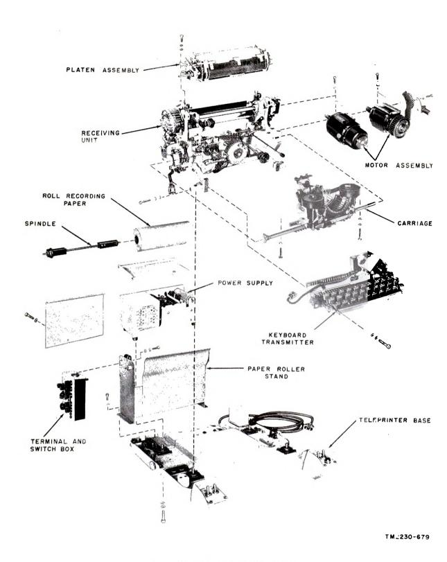
Figure 100. Teleprinter, functional groups.
