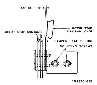
Figure 234. Motor stop switch assembly bracket adjustment.
