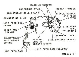
Figure 217. Line feed, line feed bell crank, and line feed detent adjustments.
