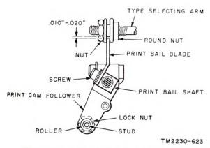
Figure 225. Printing bail blade adjustment.
