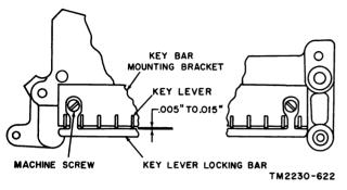
Figure 235. Key lever locking bar adjustment.
