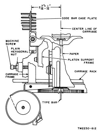
Figure 186. Carriage positioning adjustment.
