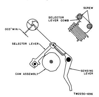
Figure 237. Selector levers and sensing levers adjustment.
