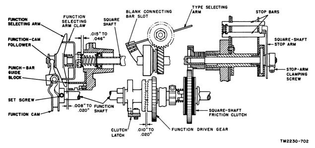
Figure 204. Function cam adjustment.
