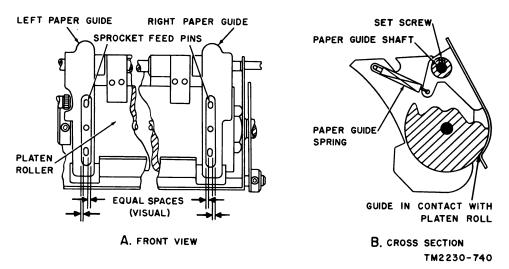
Figure 206. Paper guide alinement and adjustment.
