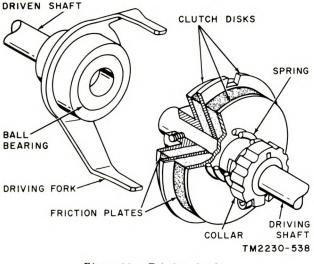
Figure 33. Friction clutch.
