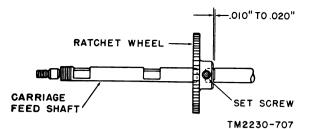
Figure 219. Carriage feed shaft ratchet wheel adjustment.
