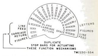
Figure 44. Characters and functions operated by stop bars.
