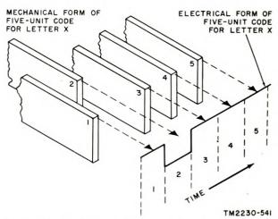
Figure 28. Relationship between mechanical and electrical forms of five-unit code.
