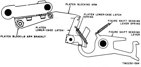
Figure 66. Platen blocking mechanism (letters position).
