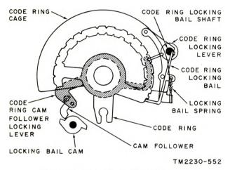
Figure 43. Code ring locking mechanism.
