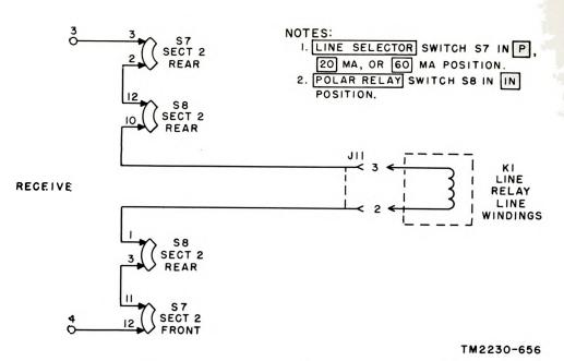
Figure 77. Teleprinter receive circuit, with line relay, ~ plified schematic.
