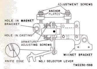
Figure 171. Armature and selector magnet bracket alinement.
