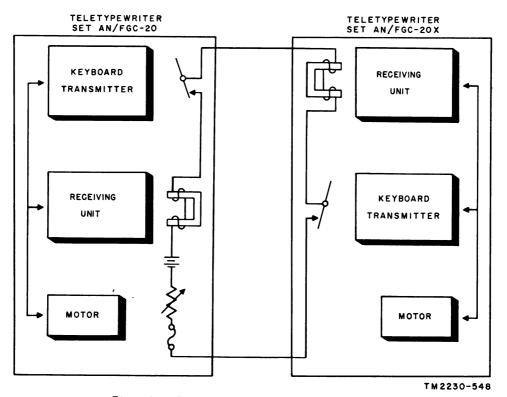
Figure 30. Interconnected teleprinters, block diagram.
