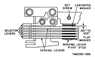
Figure 236. Sensing levers clearance alinement adjustment.
