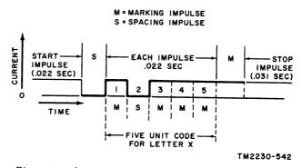
Figure 29. Standard start-stop, five-unit code signal for the letter X, plus start and stop impulses.
