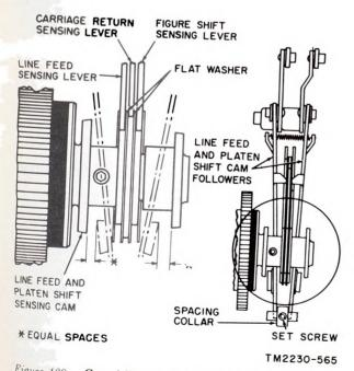
Figure 160. Cam followers and spacing collar adjustment.
