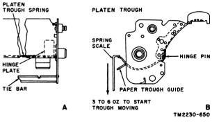
Figure 205. Platen trough spring adjustment.
