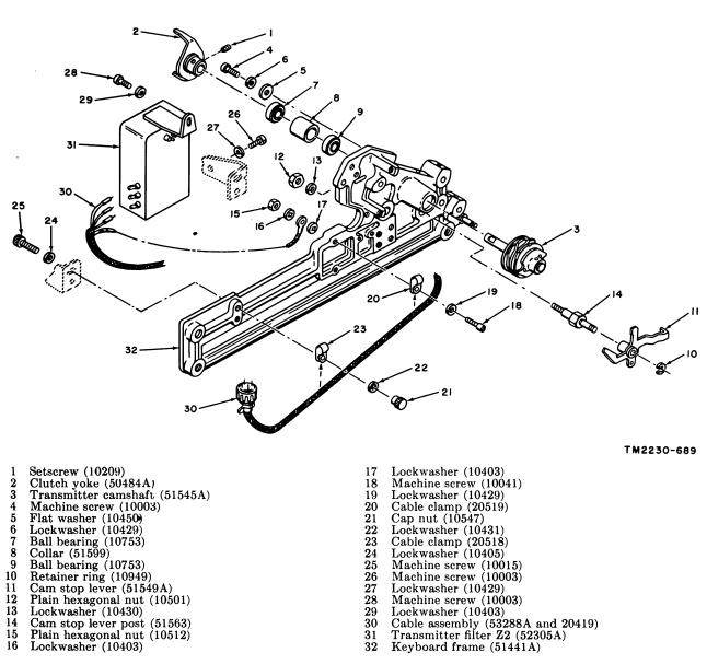
Figure 103. Transmitter camshaft and filter, exploded view.
