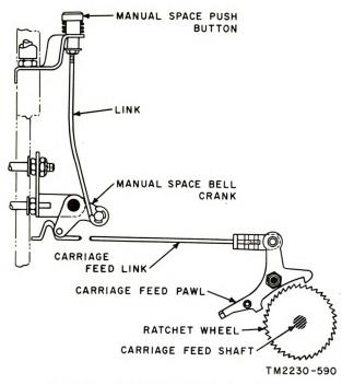
Figure 56. Manual carriage feed mechanism.
