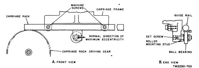
Figure 187. Ball bearing adjustment.
