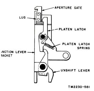
igure 65. Platen latching mechanism (letters position).
