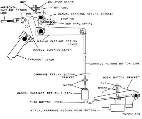
Figure 59. Manual carriage return mechanism.
