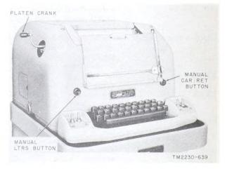
Figure 19. Teleprinter controls.
