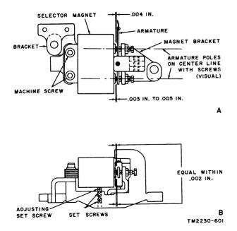
Figure 173. Selector magnet pole faces and armature alinement.
