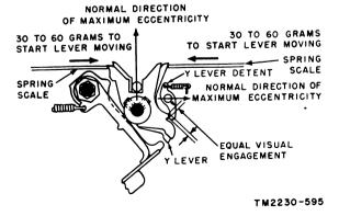
Figure 169. Y-levers detent and Y-levers adjustment.
