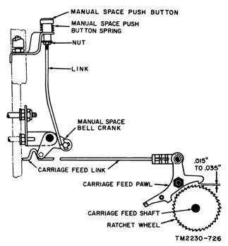
Figure 209. Manual space push button adjustment.
