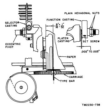
Figure 211. Platen assembly end play and positioning adjustment.
