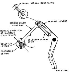
Figure 239. Sensing lever locking bail adjustment.
