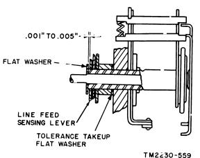
Figure 156. Sensing levers end play adjustment.
