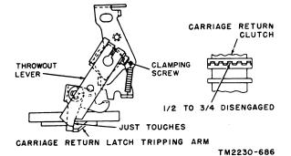
Figure 196. Throwout lever adjustment.
