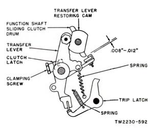
Figure 181. Function shaft clutch latch adjustment.
