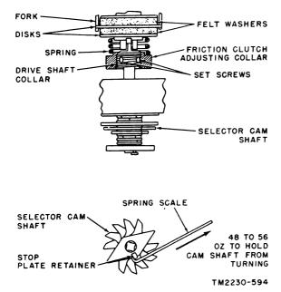
Figure 183. Selector camshaft clutch load adjustment.
