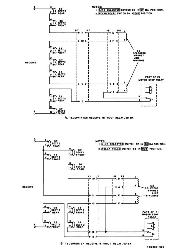
Figure 76. Teleprinter receive circuit, without line relay.
