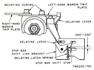
Figure 228. Left-hand margin trip plate adjustment.
