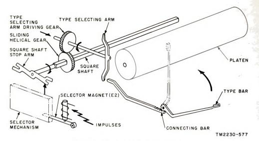
Figure 49. Typing unit basic components.
