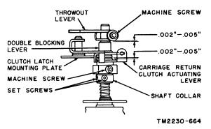
Figure 192. Carriage return clutch lever shaft cleorance adjustment.
