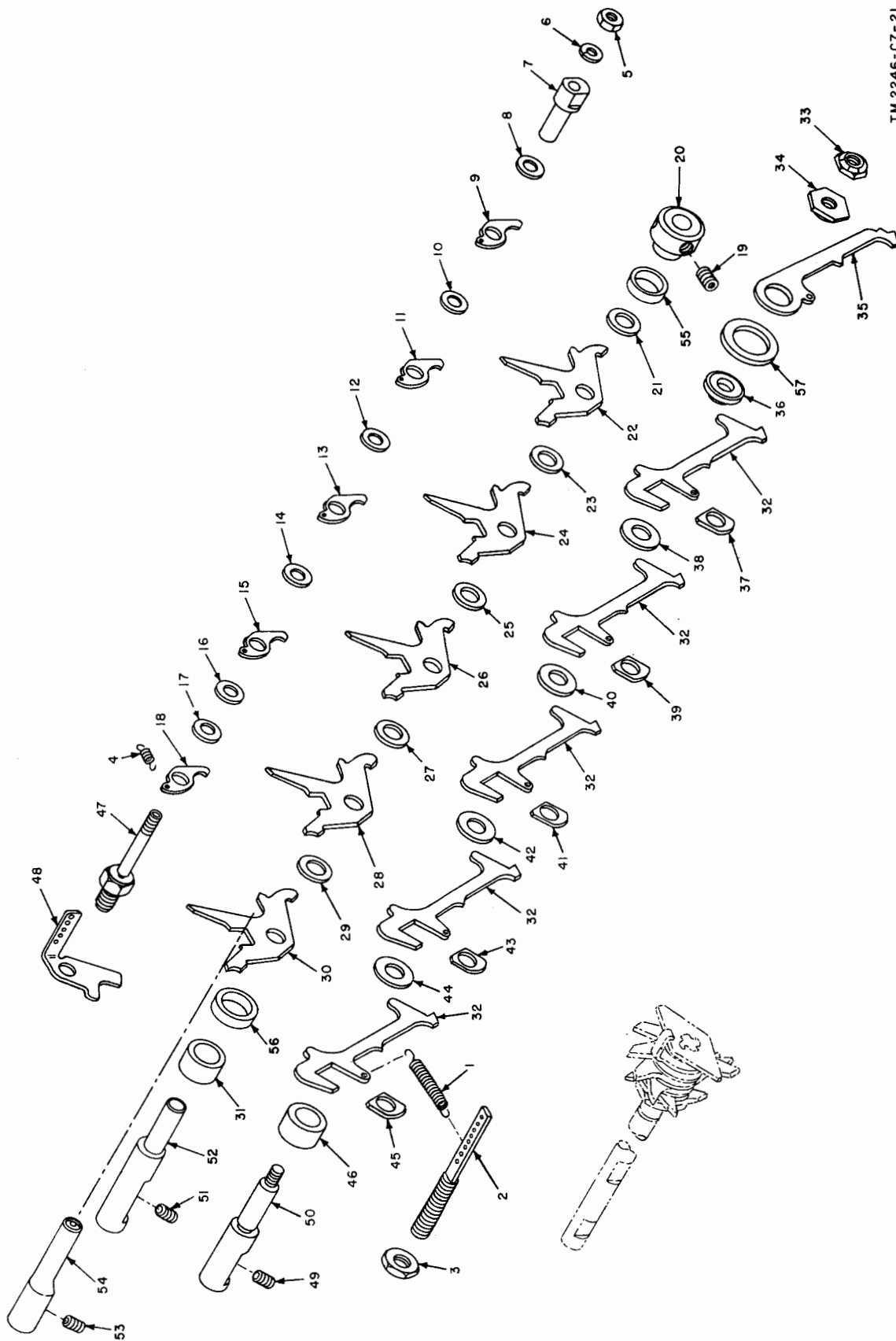
Figure 214. Selector and Y-levers, exploded view. (Superseded)
