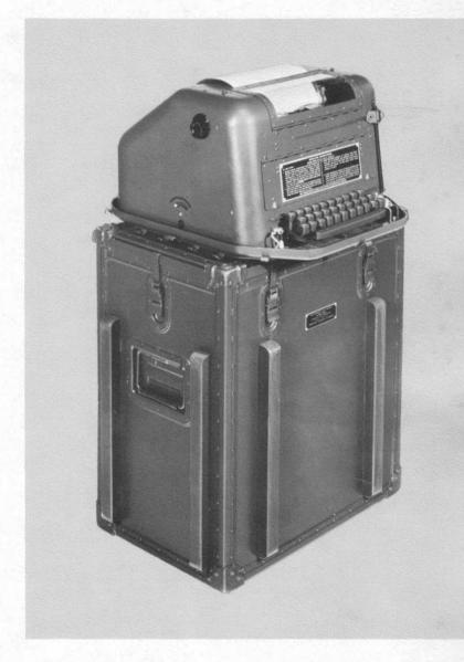
or more equipments can be interconnected, for operation with each other without the need for intermediate line modifying equipment. The TT-4C/TG features figures "H" motor stop and figures "S" signal bell. It also includes a line break switch, signal line current adjustment, and a manual carriage positioning knob. It includes a waterproof cover which, when latched in places, makes the unit buoyant in water.
