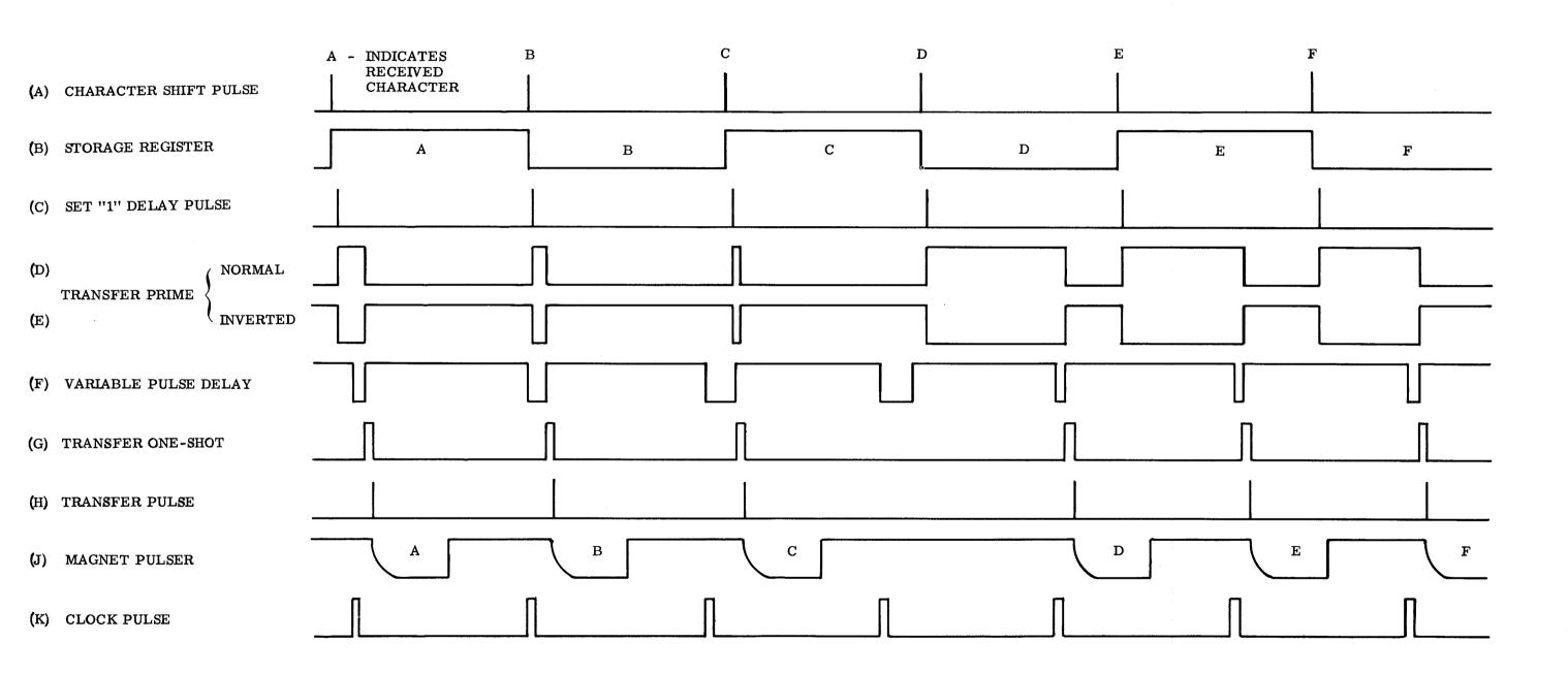
Figure 7 - Transfer Circuitry Timing Diagram, Several Cycles of Operation
