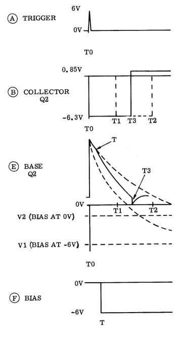
(C) Variable Delay Waveforms, Variable Bias Condition
