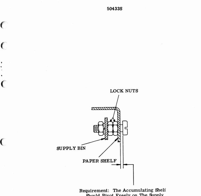
Should Pivot Freely on The Supply Bin. There Should Be Approximately 1/64 Inch Clearance.
