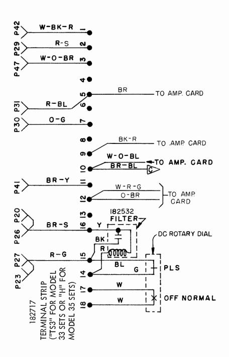
FIGURE 1. DC ROTARY DIAL CONNECTIONS
