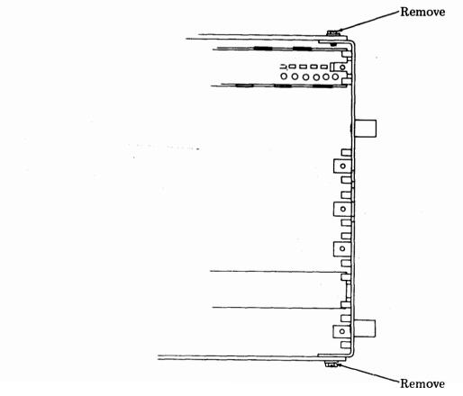
Fig. 33-Right Side Frame Removal
