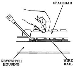
Fig. 38—Spacebar Removal
