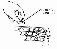
Fig. 44-Lower Plunger Removal
