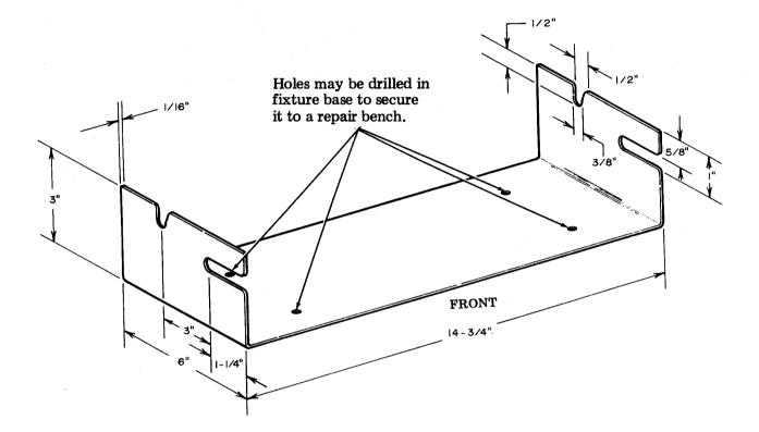
Fig. 54-Holding Fixture For High Volume Keyboard Repair
