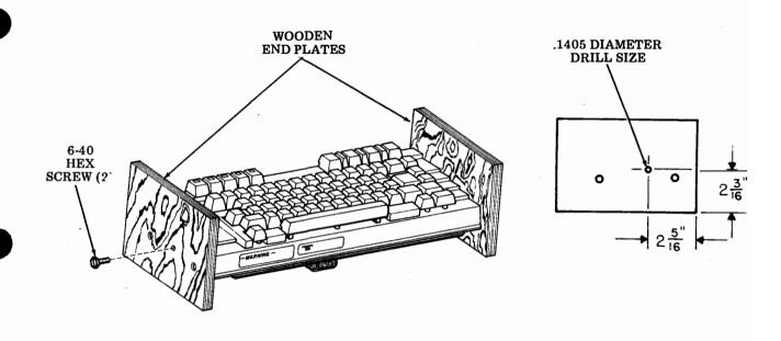
Fig. 53-Holding Fixture For Low Volume Keyboard Repair
