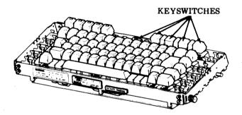
Fig. 19-Keyswitch Identification
