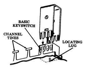
Fig. 18-Keyswitch Removal
