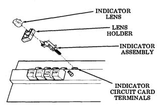
Fig. 41–Indicator Keytop Removal
