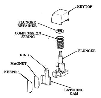
Fig. 46-Latching Keyswitch Removal
