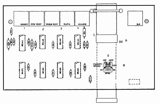
Fig. 37-Component Identification - 43K001 RO Keyboard
