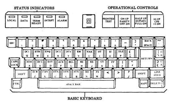
Fig. 3 –43K101/CAB or 50K122/AAF Keyboard Used in 42/43 Basic Terminal With Terminal Auxiliary Unit
