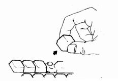
Fig. 11-Control Keytop Removal
