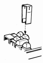
Fig. 10-Data Keytop Removal
