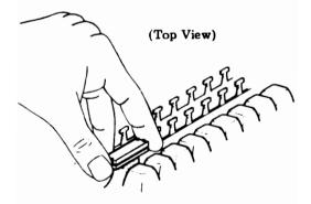
Fig. 27-Cable Connector Removal
