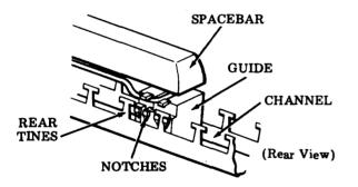
Fig. 3–Spacebar Removal
