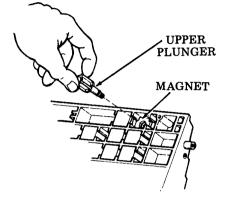
Fig. 45–Upper Plunger Removal
