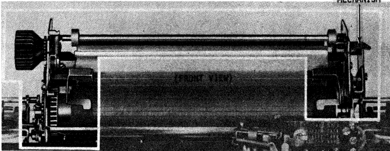
FIGURE 4-7 PAPER FEED MECHANISM
