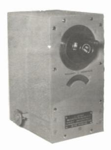
A portable, general purpose, self-contained and pre-calibrated frequency measuring cavity of the transmission type designed to measure the frequency of radio frequency signals in the range from 32,000 to 39,000 megacycles per second.
