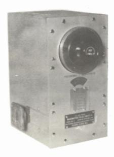
A portable, general purpose, self-contained and pre-calibrated frequency measuring cavity of the transmission type designed to measure the frequency of radio frequency signals in the range from 10,000 to 12,400 megacycles per second.
