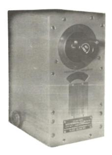
A portable, general purpose, self-contained and pre-calibrated frequency measuring cavity of the transmission type designed to measure the frequency of radio frequency signals in the range from 18,000 to 22,000 megacycles per second.
