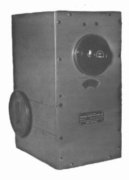
A portable, general purpose, self-contained and precalibrated coaxial line cavity of the transmission type designed to measure the frequency of radio frequency signals.
