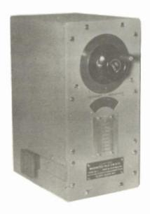
A portable, general purpose, self-contained and pre-calibrated frequency measuring cavity of the absorption type designed to measure the frequency of radio frequency signals in the range from 15,000 to 18,000 megacycles per second.
