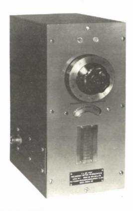
A portable, general purpose, self-contained and pre-calibrated coaxial line cavity of the transmission type designed to measure the frequency of radio frequency signals.
