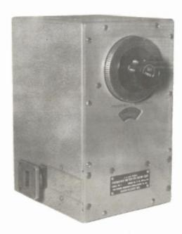
A portable, general purpose, self-contained and pre-calibrated frequency measuring cavity of the transmission type designed to measure the frequency of radio frequency signals in the range from 8200 to 10,000 megacycles per second.
