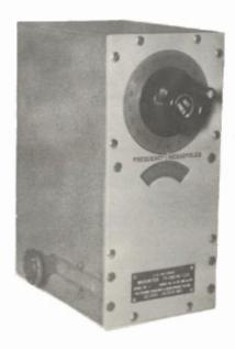
A portable, general purpose, self-contained and pre-calibrated frequency measuring cavity of the transmission type designed to measure the frequency of radio frequency signals in the range from 22,000 to 26,500 megacycles per second.
