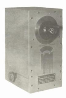
A portable, general purpose, self-contained and pre-calibrated frequency measuring cavity of the absorption type designed to measure the frequency of radio frequency signals in the range from 18,000 to 22,000 megacycles per second.
