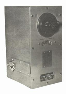
A portable, general purpose, self-contained and pre-calibrated coaxial line cavity of the transmission type designed to measure the frequency of radio frequency signals in the range from 2400 to 3950 megacycles per second.
