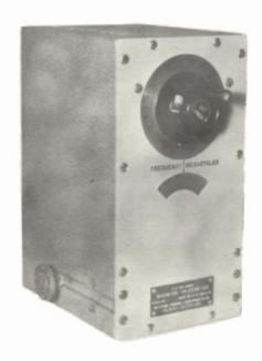
A portable, general purpose, self-contained and pre-calibrated frequency measuring cavity of the transmission type designed to measure the frequency of radio frequency signals in the range from 26,500 to 32,000 megacycles per second.
