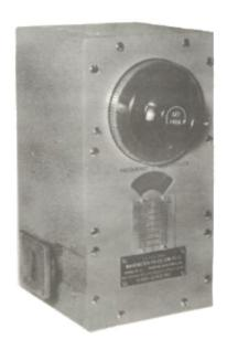
A portable, general purpose, self-contained and pre-calibrated frequency measuring cavity of the absorption type designed to measure the frequency of radio frequency signals in the range from 10,000 to 12,400 megacycles per second.
