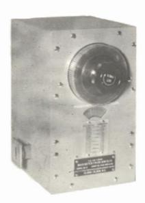
A portable, general purpose, self-contained and pre-calibrated frequency measuring cavity of the transmission type designed to measure the frequency of radio frequency signals in the range from 12,400 to 15,000 megacycles per second.
