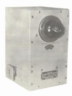
A portable, general purpose, self-contained and pre-calibrated frequency measuring cavity of the absorption type designed to measure the frequency of radio frequency signals in the range from 8200 to 10,000 megacycles per second.
