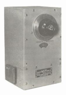
A portable, general purpose, self-contained and pre-calibrated frequency measuring cavity of the absorption type designed to measure the frequency of radio frequency signals in the range from 8200 to 10,000 megacycles per second.
