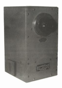
A portable, general purpose, self-contained and pre-calibrated frequency measuring cavity of the absorption type designed to measure the frequency of radio frequency signals in the range from 7050 to 8200 megacycles per second.
