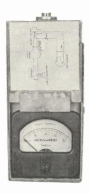
A portable, general purpose, miniature, cavity-type frequency meter used as a go-no-go check for radar beacons that operate at its frequency. Indication is on a meter dial. It is used in organizational testing.
