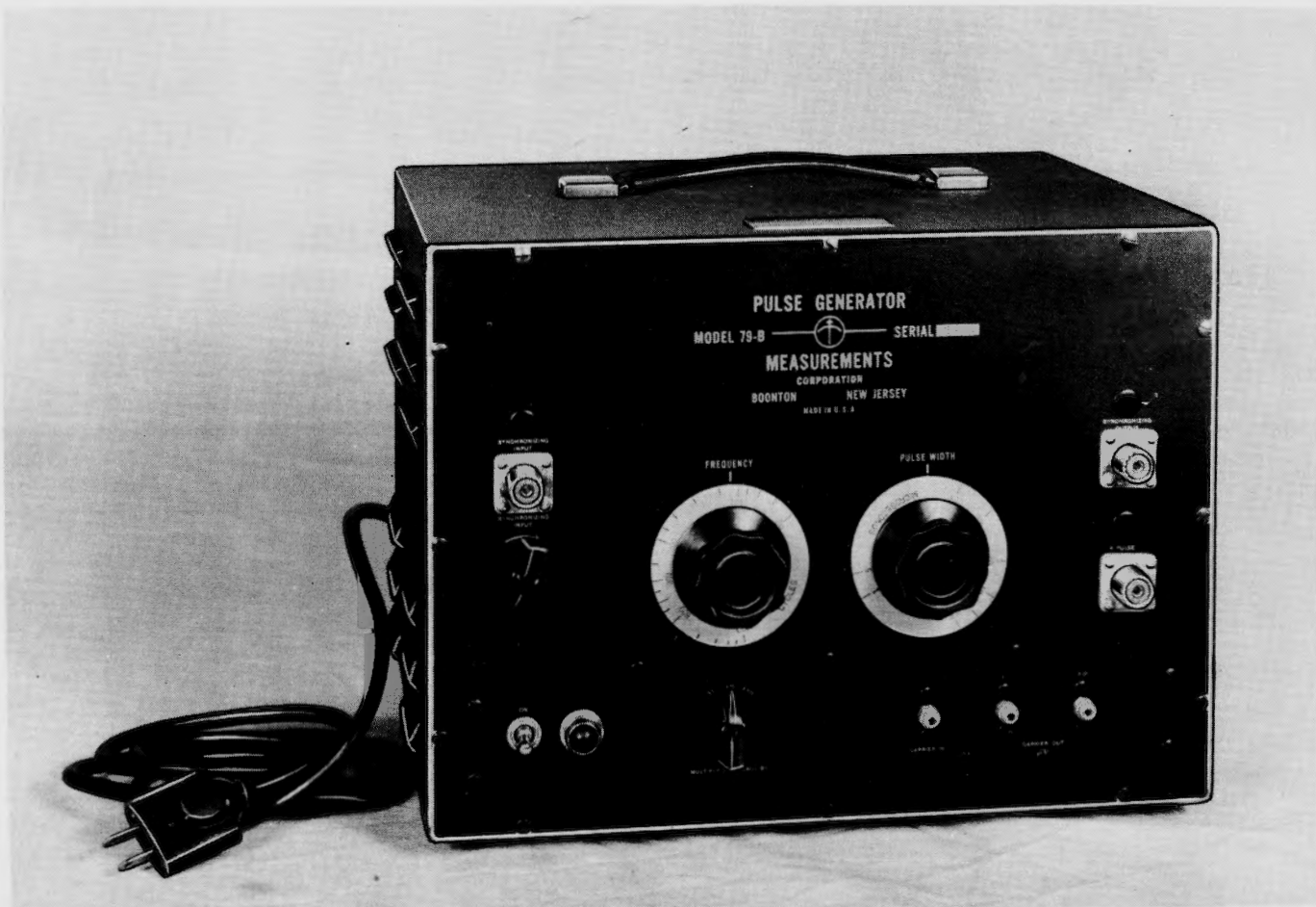
Figure 10-13. Pulse Generator—Measurements 79-B
