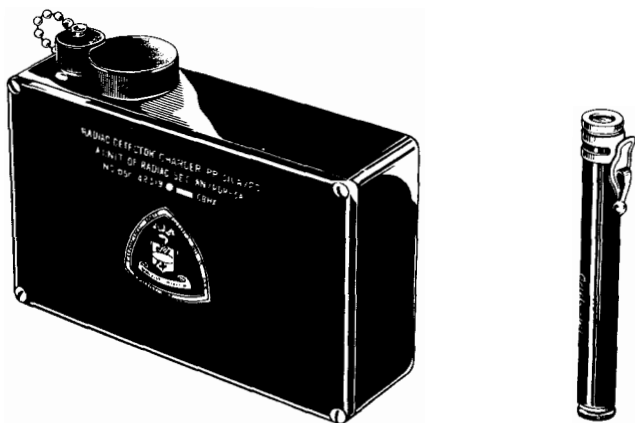
Figure 16-2.—Radiac set AN/PDR-3A.
