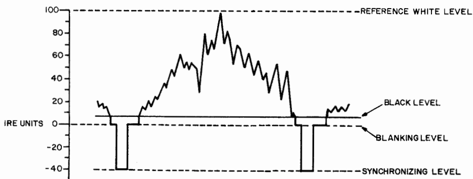
Figure 3-244. IRE Scale for Monitoring Television Signals
