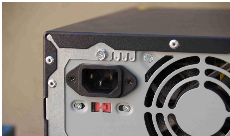
Figure 51 Computer Power Supply not in Accordance with BFG Principles
