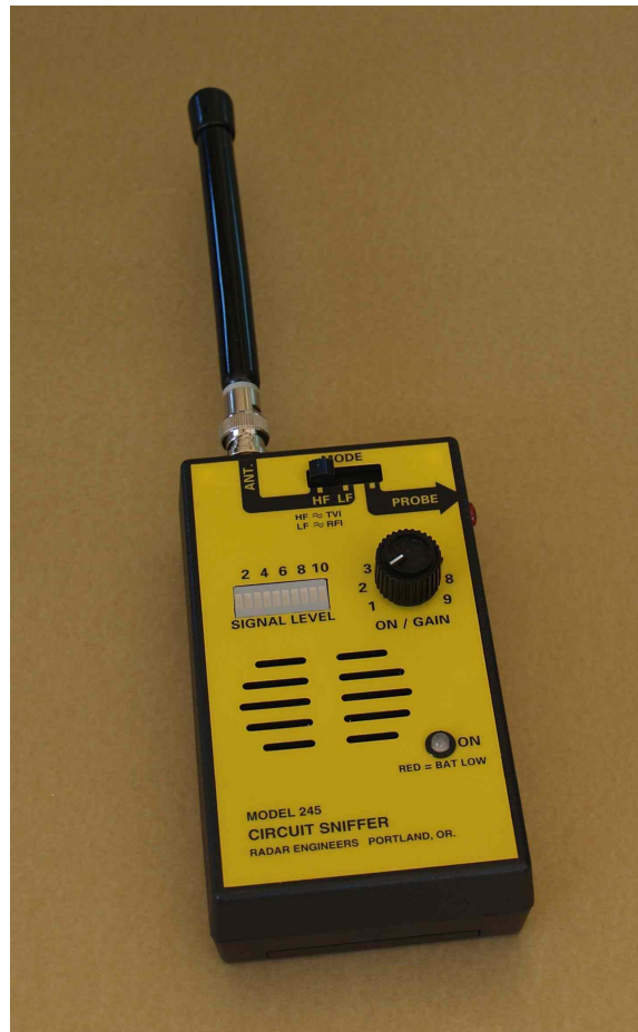
Figure 67 Circuit Sniffer Used to Locate On-Site Sources
