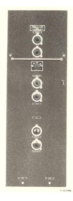
Radio Transmitter T-5( )/FRC is a long-range, high-power, medium- and low-frequency, crystal-controlled transmitting station equipment. It can be used for communication by AM (voice using additional equipment, cw, mcw, or frequency-shift keying) signals at fixed plant installations.
