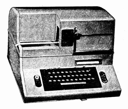
PERFORATOR-REPERFORATOR, TELETYPEWRITER TT-292/UG
