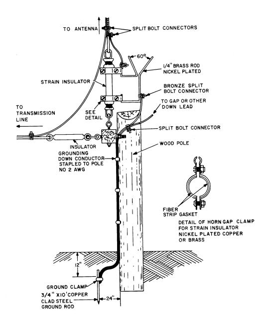
Figure 6-8. Typical Horn Gap Arrangement for Antennas
