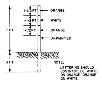
Figure 6-5. Buried Cable Marker
