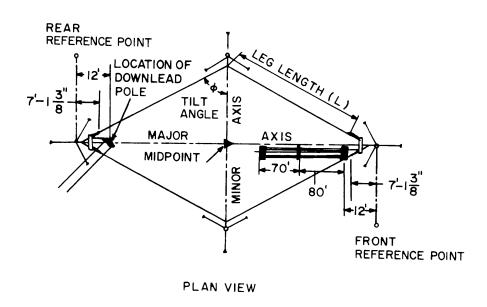
Figure 6-6. Typical Dissipation Line Arrangement
