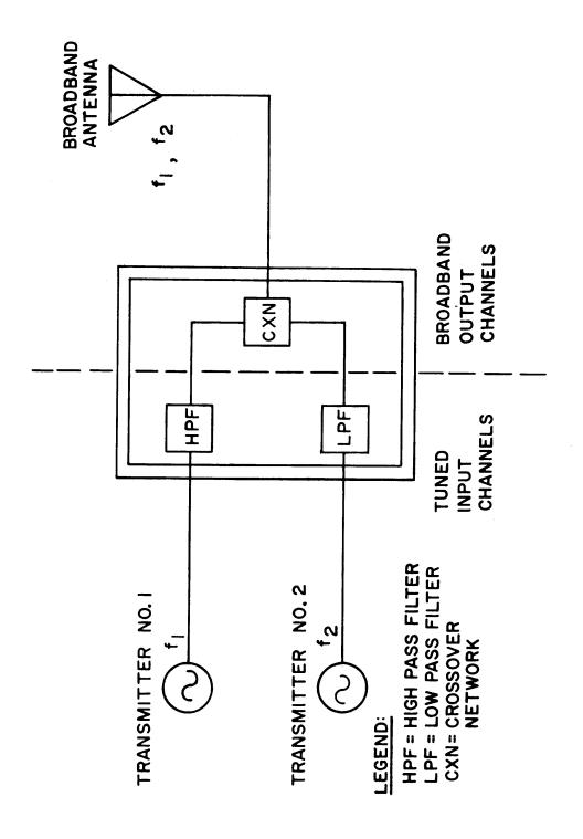
Figure 6-9. Typical Transmitting Multicoupler Arrangement
