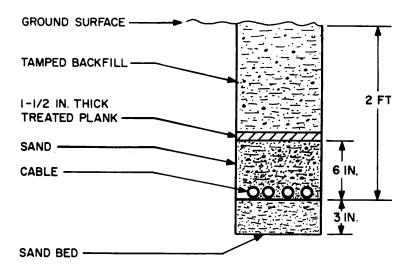
Figure 6-4. Cable Trench Layout
