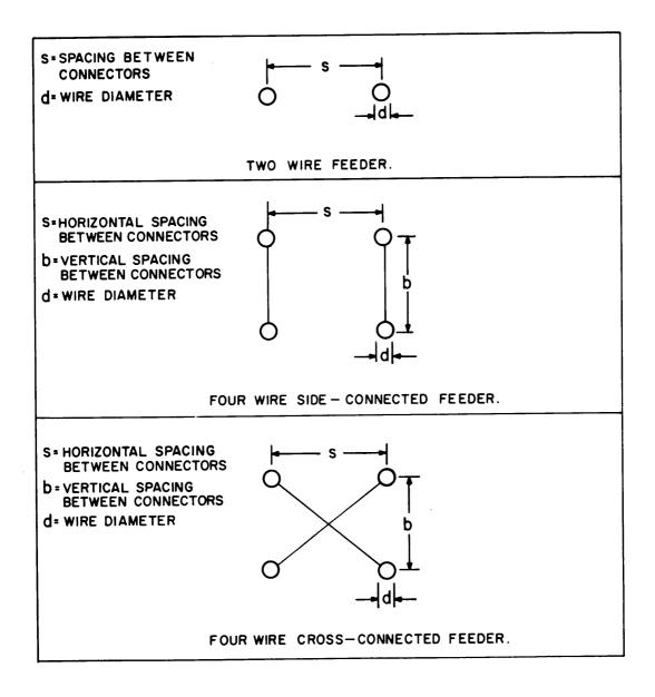
Figure 6-1. Open-Wire Transmission Line Configurations
