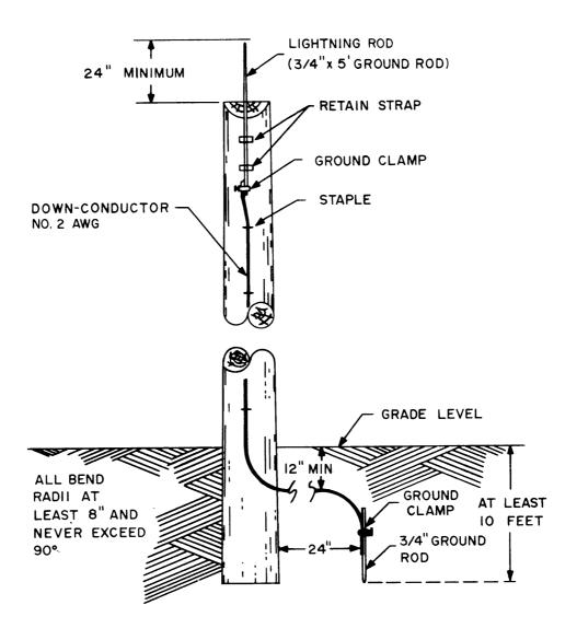
Figure 6-7. Typical Lightning Rod and Down-Conductor Arrangement
