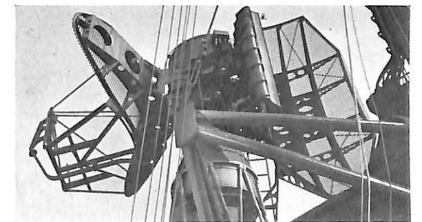
FIGURE 1—SX Antenna—Search Array, Left, Height Array, Right.
