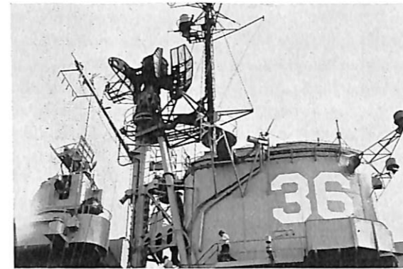
FIGURE 3—SX antenna on the U.S.S. ANTIETAM (CV-36).
