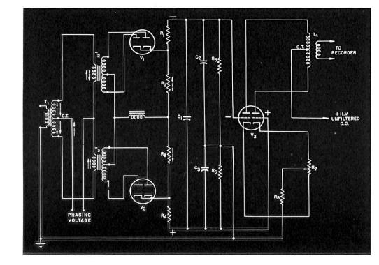
FIGURE 6-Simplified schematic diagram of discriminator.
