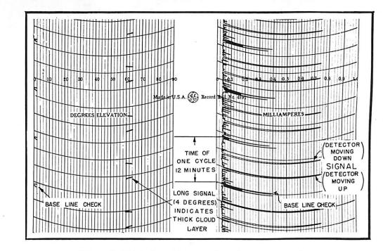
FIGURE 7-Typical graphs made by ceilometer recorder.
