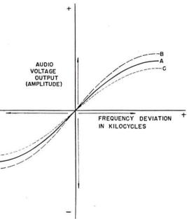
FIGURE 2-Characteristic curves for standard discriminator circuit. Curve A represents standard i-f signal amplitude; curves B and C show the effects of changing the magnitude of i signal.
