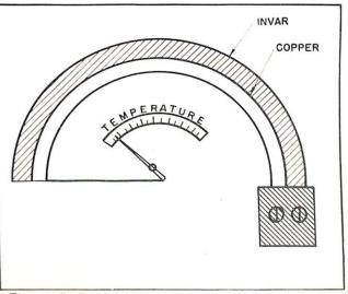
FIGURE 7-Principle of bimetallic thermometer.
