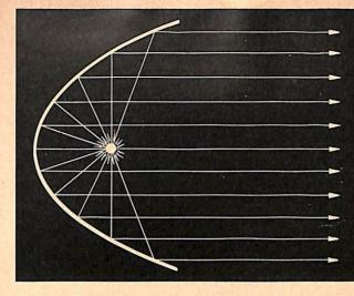
FIGURE 3-Action of a parabolic reflector and a point source of light located at the focal point.
