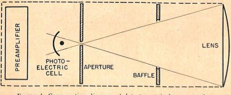
FIGURE 4-Cross section diagram of detector optical system and p-e cell.
