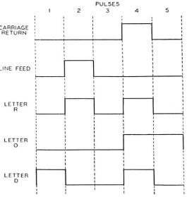
FIGURE 1-Teletypewriter codes are built up from the presence or absence of a pulse in five intervals between start and stop pulses marking the beginning and end of each code. The codes for carriage return, line feed, and the letters R, O, and D are shown above.
