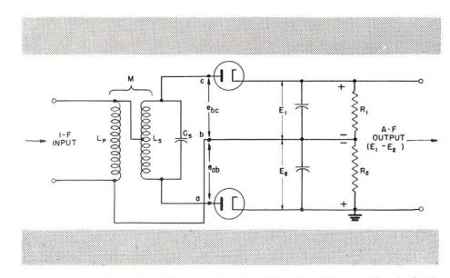
FIGURE 1-Standard discriminator circuit. This circuit is sensitive to both AM and FM and must therefore be preceded by a limiter circuit.
