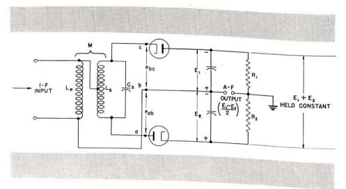
FIGURE 3-The Ratio Detector. Note similarity to standard discriminator shown in figure 1. This circuit is frequencysensitive, but substantially eliminates the AM components.
