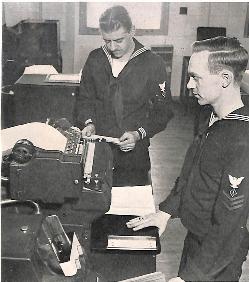
This machine automatically takes information contained in the punched cards and converts it into a complete inventory of all electronic equipment on board each ship.
