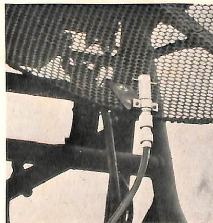
FIGURE 1 — Test dipole mounted on Mark 28 dish. Note method of making and mounting holding clamp.
