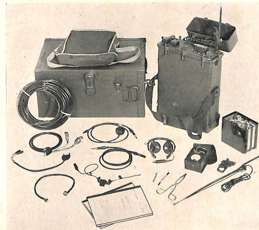
Complete MAW equipment, with extension cable, battery case, headphones, microphone, test meter, etc. Shipping chest is in background.
